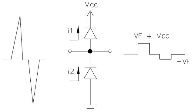
**Figure 1 - "Rail-To-Rail" Protection Topology (First Approximation)**
