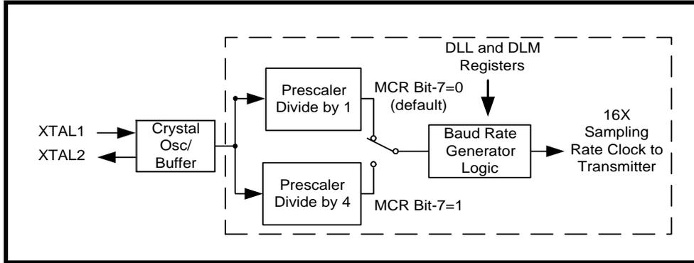
Programming the Baud Rate Generator Registers DLM and DLL provides the capability of selecting the operating data rate. **Table 3** shows the standard data rates available with a 14.7456 MHz crystal or external clock at 16X sampling rate clock rate. When using a non-standard data rate crystal or external clock, the divisor value can be calculated for DLL/DLM with the following equation.
