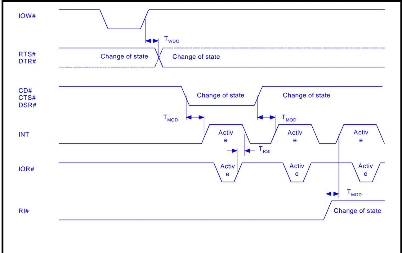
FIGURE 14. 16 MODE (INTEL) DATA BUS READ TIMING
