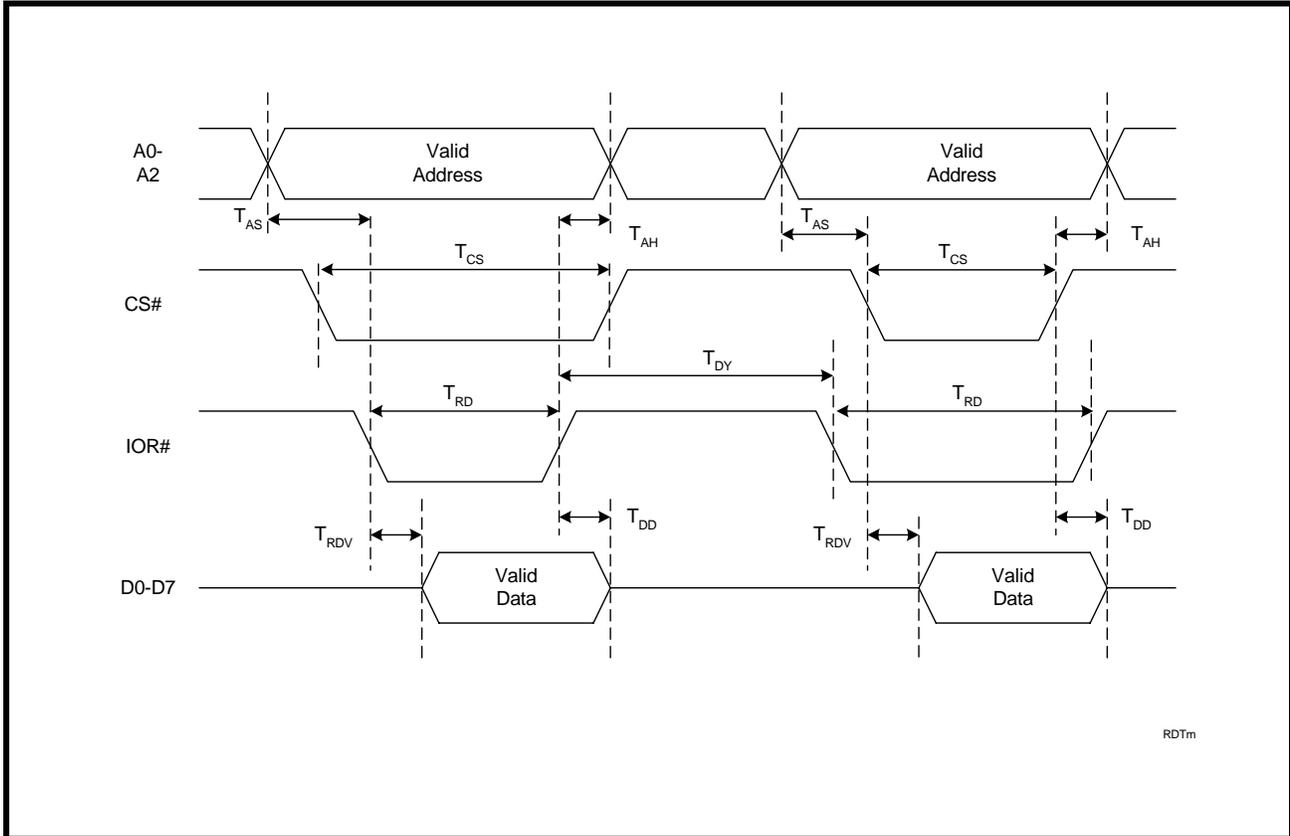
FIGURE 15. 16 MODE (INTEL) DATA BUS WRITE TIMING
