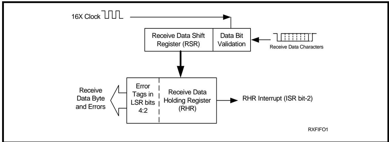
**FIGURE 9. RECEIVER OPERATION IN FIFO AND AUTO RTS FLOW CONTROL MODE**
