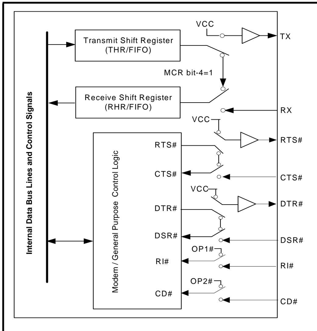
**SINGLE CHANNEL INTEGRATED UART AND RS-232 TRANSCEIVER**
