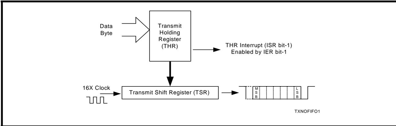
**2.10.3 Transmitter Operation in FIFO Mode**
