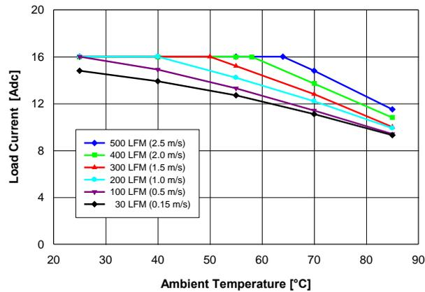
Fig. 5.0V.1: Available load current vs. ambient temperature and airflow rates for  $V_{out} = 5.0\text{ V}$  converter mounted vertically with  $V_{in} = 12\text{ V}$ , and maximum MOSFET temperature  $\leq 120\text{ }^\circ\text{C}$ .
