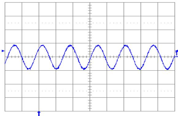
Fig. 5.0V.5: Output voltage ripple (20 mV/div.) at full rated load current into a resistive load with external capacitance  $100\text{ }\mu\text{F}$  ceramic and  $V_{in} = 12\text{ V}$  for  $V_{out} = 5.0\text{ V}$ . Time scale: 2  $\mu\text{s}$ /div.
