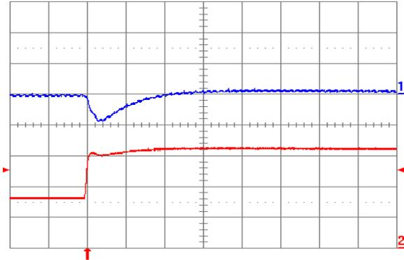
Fig. 1.2V.6: Output voltage response for  $V_{out} = 1.2\text{ V}$  to positive load current step change from 8 A to 16 A with slew rate of  $5\text{ A}/\mu\text{s}$  at  $V_{in} = 12\text{ V}$ . Top trace: output voltage (200 mV/div.); Bottom trace: load current (5 A/div.).  $C_o = 100\text{ }\mu\text{F}$  ceramic. Time scale:  $20\text{ }\mu\text{s}/\text{div}$ .
