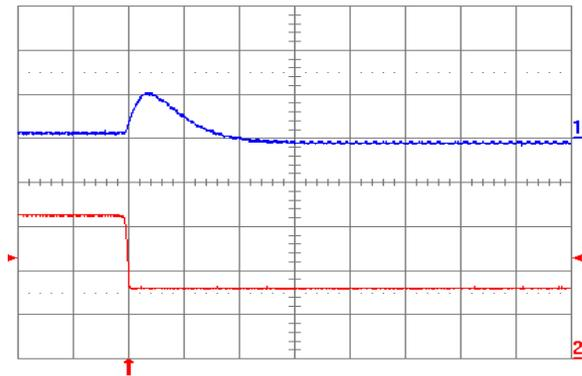
Fig. 1.0V.7: Output voltage response for  $V_{out} = 1.0\text{ V}$  to negative load current step change from  $16\text{ A}$  to  $8\text{ A}$  with slew rate of  $-5\text{ A}/\mu\text{s}$  at  $V_{in} = 12\text{ V}$ . Top trace: output voltage ( $200\text{ mV/div.}$ ); Bottom trace: load current ( $5\text{ A/div.}$ ).  $C_o = 100\ \mu\text{F}$  ceramic. Time scale:  $20\ \mu\text{s/div.}$
