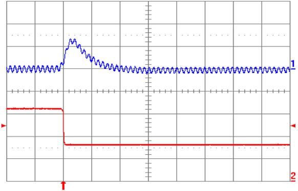
Fig. 5.0V.7: Output voltage response for  $V_{out} = 5.0\text{ V}$  to negative load current step change from 16 A to 8 A with slew rate of  $-5\text{ A}/\mu\text{s}$  at  $V_{in} = 12\text{ V}$ . Top trace: output voltage (200 mV/div.); Bottom trace: load current (5 A/div.).  $C_o = 100\text{ }\mu\text{F}$  ceramic. Time scale:  $20\text{ }\mu\text{s}/\text{div}$ .
