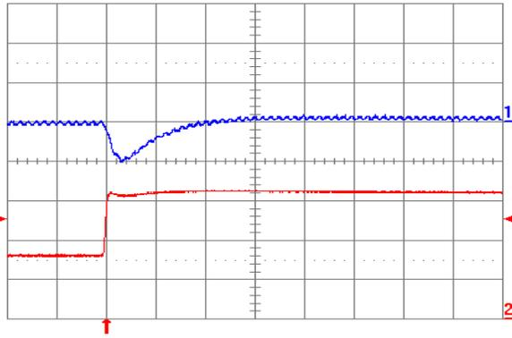
Fig. 1.8V.6: Output voltage response for  $V_{out} = 1.8\text{ V}$  to positive load current step change from  $8\text{ A}$  to  $16\text{ A}$  with slew rate of  $5\text{ A}/\mu\text{s}$  at  $V_{in} = 12\text{ V}$ . Top trace: output voltage ( $200\text{ mV/div.}$ ); Bottom trace: load current ( $5\text{ A/div.}$ ).  $C_o = 100\ \mu\text{F}$  ceramic. Time scale:  $20\ \mu\text{s/div.}$
