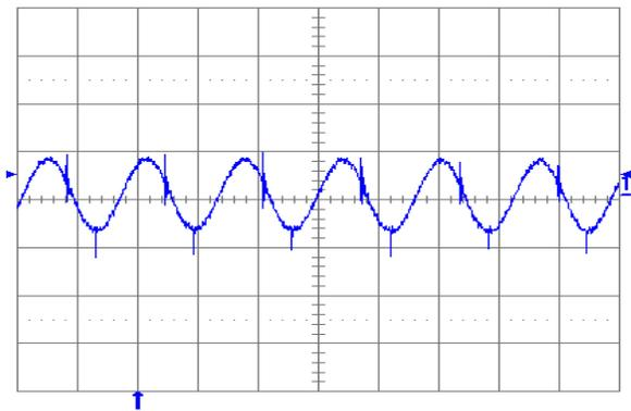
Fig. 3.3V.5: Output voltage ripple ( $20\text{ mV/div.}$ ) at full rated load current into a resistive load with external capacitance  $100\ \mu\text{F}$  ceramic and  $V_{in} = 12\text{ V}$  for  $V_{out} = 3.3\text{ V}$ . Time scale:  $2\ \mu\text{s/div.}$
