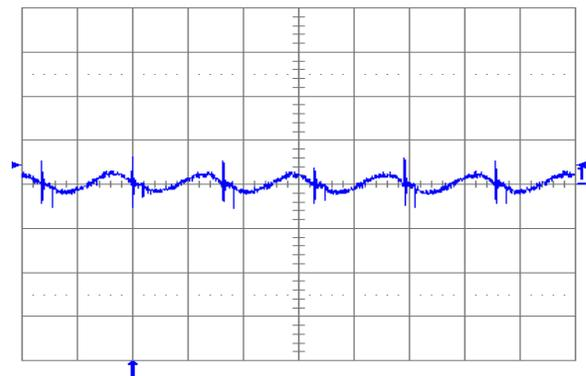
Fig. 1.2V.5: Output voltage ripple (20 mV/div.) at full rated load current into a resistive load with external capacitance  $100\text{ }\mu\text{F}$  ceramic and  $V_{in} = 12\text{ V}$  for  $V_{out} = 1.2\text{ V}$ . Time scale: 2  $\mu\text{s}$ /div.
