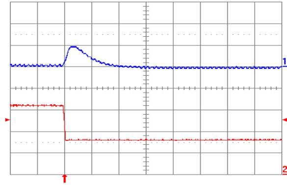
Fig. 1.8V.7: Output voltage response for  $V_{out} = 1.8\text{ V}$  to negative load current step change from  $16\text{ A}$  to  $8\text{ A}$  with slew rate of  $-5\text{ A}/\mu\text{s}$  at  $V_{in} = 12\text{ V}$ . Top trace: output voltage ( $200\text{ mV/div.}$ ); Bottom trace: load current ( $5\text{ A/div.}$ ).  $C_o = 100\ \mu\text{F}$  ceramic. Time scale:  $20\ \mu\text{s/div.}$
