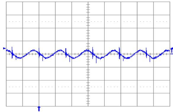
Fig. 1.5V.5: Output voltage ripple (20 mV/div.) at full rated load current into a resistive load with external capacitance  $100\text{ }\mu\text{F}$  ceramic and  $V_{in} = 12\text{ V}$  for  $V_{out} = 1.5\text{ V}$ . Time scale: 2  $\mu\text{s}$ /div.
