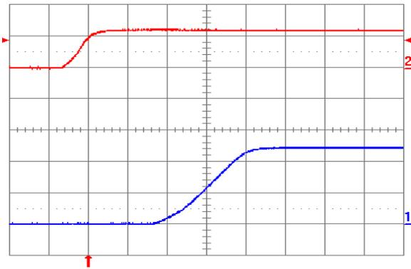
Fig. 2.5V.4: Turn-on transient for  $V_{out} = 2.5\text{ V}$  with application of  $V_{in}$  at full rated load current (resistive) and  $100\text{ }\mu\text{F}$  external capacitance at  $V_{in} = 12\text{ V}$ . Top trace:  $V_{in}$  (10 V/div.); Bottom trace: output voltage (1 V/div.); Time scale: 2 ms/div.
