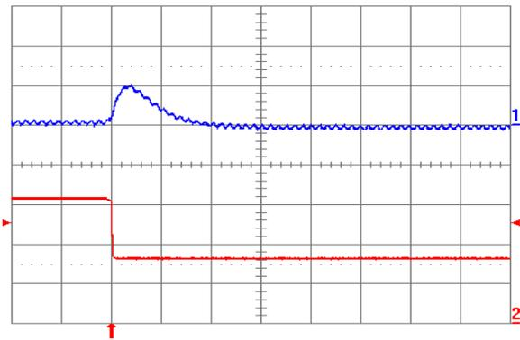
Fig. 2.5V.7: Output voltage response for  $V_{out} = 2.5\text{ V}$  to negative load current step change from 16 A to 8 A with slew rate of  $-5\text{ A}/\mu\text{s}$  at  $V_{in} = 12\text{ V}$ . Top trace: output voltage (200 mV/div.); Bottom trace: load current (5 A/div.).  $C_o = 100\text{ }\mu\text{F}$  ceramic. Time scale: 20  $\mu\text{s}$ /div.
