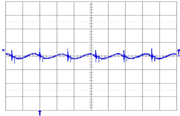
Fig. 1.0V.5: Output voltage ripple ( $20\text{ mV/div.}$ ) at full rated load current into a resistive load with external capacitance  $100\ \mu\text{F}$  ceramic and  $V_{in} = 12\text{ V}$  for  $V_{out} = 1.0\text{ V}$ . Time scale:  $2\ \mu\text{s/div.}$
