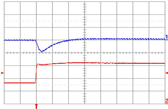
Fig. 1.5V.6: Output voltage response for  $V_{out} = 1.5\text{ V}$  to positive load current step change from 8 A to 16 A with slew rate of  $5\text{ A}/\mu\text{s}$  at  $V_{in} = 12\text{ V}$ . Top trace: output voltage (200 mV/div.); Bottom trace: load current (5 A/div.).  $C_o = 100\text{ }\mu\text{F}$  ceramic. Time scale: 20  $\mu\text{s}$ /div.
