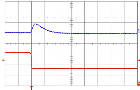
Fig. 1.5V.7: Output voltage response for  $V_{out} = 1.5\text{ V}$  to negative load current step change from 16 A to 8 A with slew rate of  $-5\text{ A}/\mu\text{s}$  at  $V_{in} = 12\text{ V}$ . Top trace: output voltage (200 mV/div.); Bottom trace: load current (5 A/div.).  $C_o = 100\text{ }\mu\text{F}$  ceramic. Time scale: 20  $\mu\text{s}$ /div.
