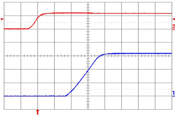
Fig. 3.3V.4: Turn-on transient for  $V_{out} = 3.3\text{ V}$  with application of  $V_{in}$  at full rated load current (resistive) and  $100\ \mu\text{F}$  external capacitance at  $V_{in} = 12\text{ V}$ . Top trace:  $V_{in}$  ( $10\text{ V/div.}$ ); Bottom trace: output voltage ( $1\text{ V/div.}$ ); Time scale:  $2\text{ ms/div.}$
