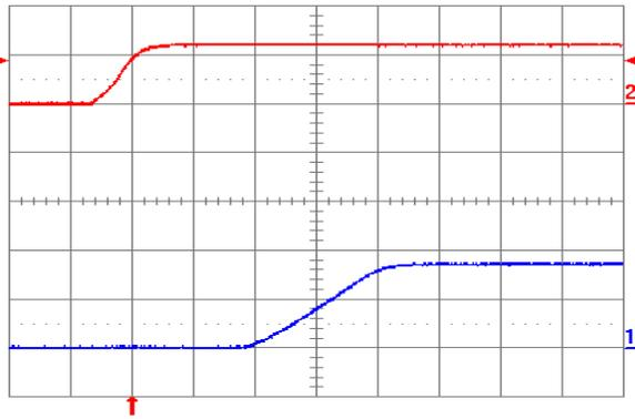
Fig. 1.8V.4: Turn-on transient for  $V_{out} = 1.8\text{ V}$  with application of  $V_{in}$  at full rated load current (resistive) and  $100\ \mu\text{F}$  external capacitance at  $V_{in} = 12\text{ V}$ . Top trace:  $V_{in}$  ( $10\text{ V/div.}$ ); Bottom trace: output voltage ( $1\text{ V/div.}$ ); Time scale:  $2\text{ ms/div.}$
