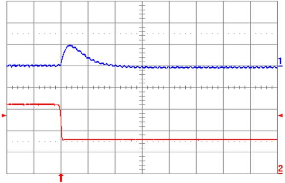
Fig. 2.0V.7: Output voltage response for  $V_{out} = 2.0\text{ V}$  to negative load current step change from 16 A to 8 A with slew rate of  $-5\text{ A}/\mu\text{s}$  at  $V_{in} = 12\text{ V}$ . Top trace: output voltage (200 mV/div.); Bottom trace: load current (5 A/div.).  $C_o = 100\ \mu\text{F}$  ceramic. Time scale:  $20\ \mu\text{s}/\text{div}$ .
