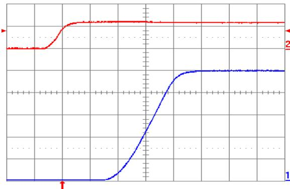
Fig. 5.0V.4: Turn-on transient for  $V_{out} = 5.0\text{ V}$  with application of  $V_{in}$  at full rated load current (resistive) and  $100\text{ }\mu\text{F}$  external capacitance at  $V_{in} = 12\text{ V}$ . Top trace:  $V_{in}$  (10 V/div.); Bottom trace: output voltage (1 V/div.); Time scale: 2 ms/div.
