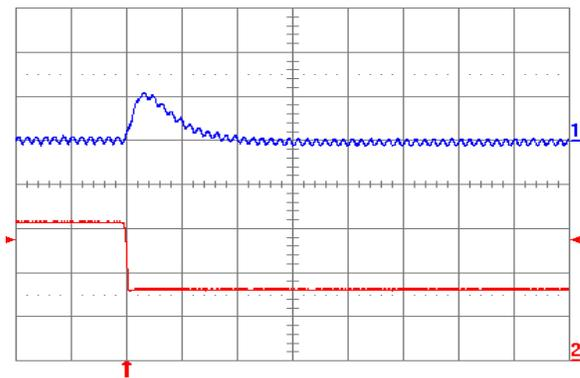
Fig. 3.3V.7: Output voltage response for  $V_{out} = 3.3\text{ V}$  to negative load current step change from  $16\text{ A}$  to  $8\text{ A}$  with slew rate of  $-5\text{ A}/\mu\text{s}$  at  $V_{in} = 12\text{ V}$ . Top trace: output voltage ( $200\text{ mV/div.}$ ); Bottom trace: load current ( $5\text{ A/div.}$ ).  $C_o = 100\ \mu\text{F}$  ceramic. Time scale:  $20\ \mu\text{s/div.}$
