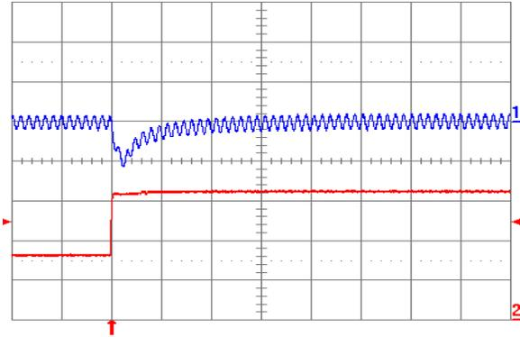
Fig. 5.0V.6: Output voltage response for  $V_{out} = 5.0\text{ V}$  to positive load current step change from 8A to 16A with slew rate of  $5\text{ A}/\mu\text{s}$  at  $V_{in} = 12\text{ V}$ . Top trace: output voltage (200 mV/div.); Bottom trace: load current (5 A/div.).  $C_o = 100\text{ }\mu\text{F}$  ceramic. Time scale:  $20\text{ }\mu\text{s}/\text{div}$ .
