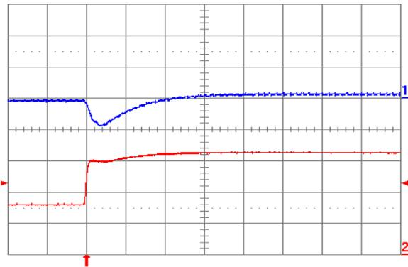
Fig. 1.0V.6: Output voltage response for  $V_{out} = 1.0\text{ V}$  to positive load current step change from  $8\text{ A}$  to  $16\text{ A}$  with slew rate of  $5\text{ A}/\mu\text{s}$  at  $V_{in} = 12\text{ V}$ . Top trace: output voltage ( $200\text{ mV/div.}$ ); Bottom trace: load current ( $5\text{ A/div.}$ ).  $C_o = 100\ \mu\text{F}$  ceramic. Time scale:  $20\ \mu\text{s/div.}$
