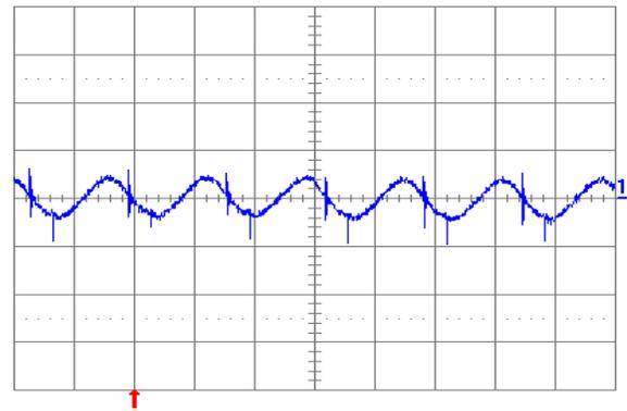
Fig. 2.5V.5: Output voltage ripple (20 mV/div.) at full rated load current into a resistive load with external capacitance  $100\text{ }\mu\text{F}$  ceramic and  $V_{in} = 12\text{ V}$  for  $V_{out} = 2.5\text{ V}$ . Time scale: 2  $\mu\text{s}$ /div.
