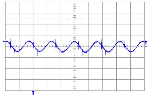
Fig. 2.0V.5: Output voltage ripple (20 mV/div.) at full rated load current into a resistive load with external capacitance  $100\text{ }\mu\text{F}$  ceramic and  $V_{in} = 12\text{ V}$  for  $V_{out} = 2.0\text{ V}$ . Time scale:  $2\text{ }\mu\text{s/div.}$
