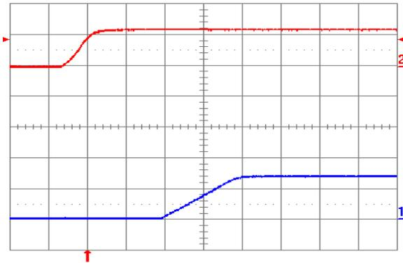
Fig. 0.7525V.4: Turn-on transient for  $V_{out} = 0.7525\text{ V}$  with application of  $V_{in}$  at full rated load current (resistive) and  $100\text{ }\mu\text{F}$  external capacitance at  $V_{in} = 12\text{ V}$ . Top trace:  $V_{in}$  (10 V/div.); Bottom trace: output voltage (0.5 V/div.); Time scale: 2 ms/div.
