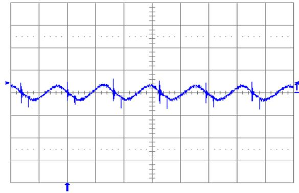
Fig. 1.8V.5: Output voltage ripple ( $20\text{ mV/div.}$ ) at full rated load current into a resistive load with external capacitance  $100\ \mu\text{F}$  ceramic and  $V_{in} = 12\text{ V}$  for  $V_{out} = 1.8\text{ V}$ . Time scale:  $2\ \mu\text{s/div.}$
