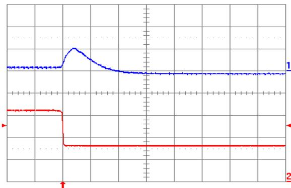
Fig. 0.7525V.7: Output voltage response for  $V_{out} = 0.7525\text{ V}$  to negative load current step change from 16 A to 8 A with slew rate of  $-5\text{ A}/\mu\text{s}$  at  $V_{in} = 12\text{ V}$ . Top trace: output voltage (200 mV/div.); Bottom trace: load current (5 A/div.).  $C_o = 100\text{ }\mu\text{F}$  ceramic. Time scale: 20  $\mu\text{s}$ /div.
