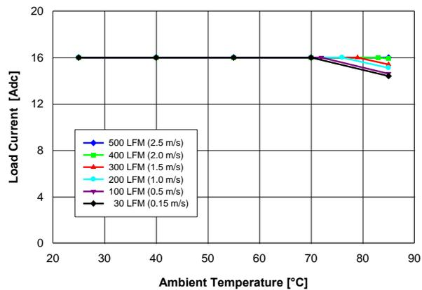
Fig. 0.7525V.1: Available load current vs. ambient temperature and airflow rates for  $V_{out} = 1.0\text{ V}$  converter mounted vertically with  $V_{in} = 12\text{ V}$ , and maximum MOSFET temperature  $\leq 120\text{ }^\circ\text{C}$ .
