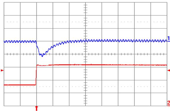
Fig. 3.3V.6: Output voltage response for  $V_{out} = 3.3\text{ V}$  to positive load current step change from  $8\text{ A}$  to  $16\text{ A}$  with slew rate of  $5\text{ A}/\mu\text{s}$  at  $V_{in} = 12\text{ V}$ . Top trace: output voltage ( $200\text{ mV/div.}$ ); Bottom trace: load current ( $5\text{ A/div.}$ ).  $C_o = 100\ \mu\text{F}$  ceramic. Time scale:  $20\ \mu\text{s/div.}$
