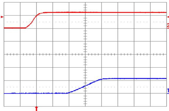
Fig. 1.2V.4: Turn-on transient for  $V_{out} = 1.2\text{ V}$  with application of  $V_{in}$  at full rated load current (resistive) and  $100\text{ }\mu\text{F}$  external capacitance at  $V_{in} = 12\text{ V}$ . Top trace:  $V_{in}$  (10V/div.); Bottom trace: output voltage (1 V/div.); Time scale: 2 ms/div.
