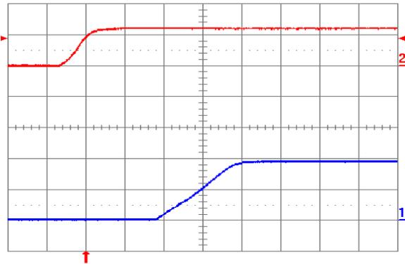
Fig. 1.0V.4: Turn-on transient for  $V_{out} = 1.0\text{ V}$  with application of  $V_{in}$  at full rated load current (resistive) and  $100\ \mu\text{F}$  external capacitance at  $V_{in} = 12\text{ V}$ . Top trace:  $V_{in}$  ( $10\text{ V/div.}$ ); Bottom trace: output voltage ( $0.5\text{ V/div.}$ ); Time scale:  $2\text{ ms/div.}$
