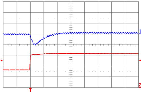
Fig. 2.5V.6: Output voltage response for  $V_{out} = 2.5\text{ V}$  to positive load current step change from 8 A to 16 A with slew rate of  $5\text{ A}/\mu\text{s}$  at  $V_{in} = 12\text{ V}$ . Top trace: output voltage (200 mV/div.); Bottom trace: load current (5 A/div.).  $C_o = 100\text{ }\mu\text{F}$  ceramic. Time scale: 20  $\mu\text{s}$ /div.
