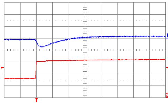
Fig. 0.7525V.6: Output voltage response for  $V_{out} = 0.7525\text{ V}$  to positive load current step change from 8 A to 16 A with slew rate of  $5\text{ A}/\mu\text{s}$  at  $V_{in} = 12\text{ V}$ . Top trace: output voltage (200 mV/div.); Bottom trace: load current (5 A/div.).  $C_o = 100\text{ }\mu\text{F}$  ceramic. Time scale: 20  $\mu\text{s}$ /div.
