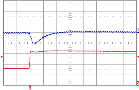
Fig. 2.0V.6: Output voltage response for  $V_{out} = 2.0\text{ V}$  to positive load current step change from 8 A to 16 A with slew rate of  $5\text{ A}/\mu\text{s}$  at  $V_{in} = 12\text{ V}$ . Top trace: output voltage (200 mV/div.); Bottom trace: load current (5 A/div.).  $C_o = 100\ \mu\text{F}$  ceramic. Time scale:  $20\ \mu\text{s}/\text{div}$ .
