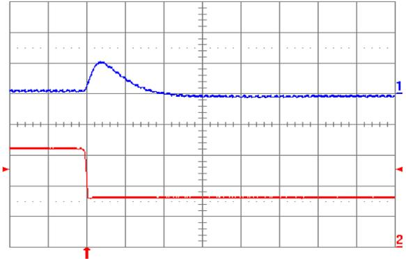
Fig. 1.2V.7: Output voltage response for  $V_{out} = 1.2\text{ V}$  to negative load current step change from 16 A to 8 A with slew rate of  $-5\text{ A}/\mu\text{s}$  at  $V_{in} = 12\text{ V}$ . Top trace: output voltage (200 mV/div.); Bottom trace: load current (5 A/div.).  $C_o = 100\text{ }\mu\text{F}$  ceramic. Time scale:  $20\text{ }\mu\text{s}/\text{div}$ .
