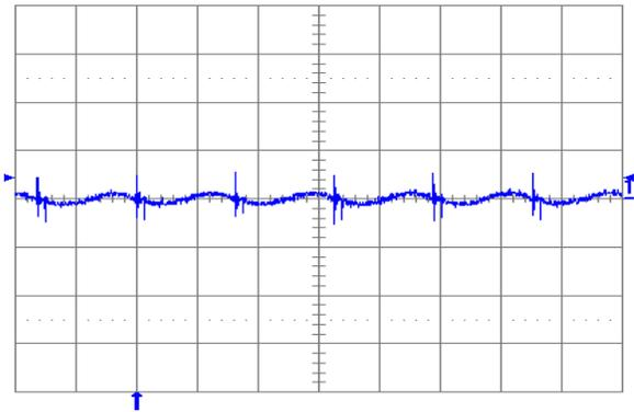
Fig. 0.7525V.5: Output voltage ripple (20 mV/div.) at full rated load current into a resistive load with external capacitance  $100\text{ }\mu\text{F}$  ceramic and  $V_{in} = 12\text{ V}$  for  $V_{out} = 0.7525\text{ V}$ . Time scale: 2  $\mu\text{s}$ /div.
