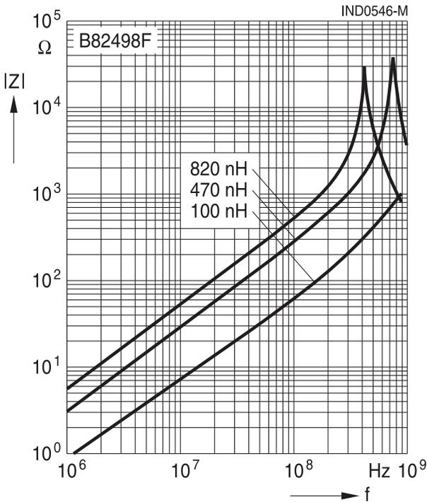
**Impedance  $|Z|$  vs. frequency  $f$  (ferrite core)**
