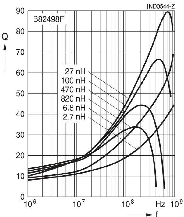
**Q factor versus frequency  $f$  (ferrite core)**
