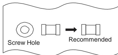
2. If you mount the capacitor near components that generate heat, take note of the heat from the other components and carefully check the self-heating of the capacitor before using.
