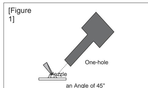
3. Optimum solder amount when re-working with a soldering iron
