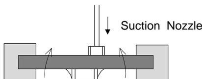
2-2. Inserting Components with Leads into Boards
