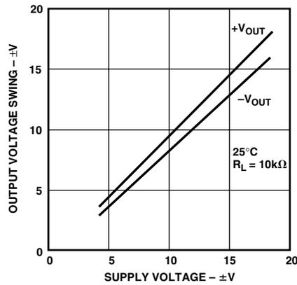
TPC 2. Output Voltage Swing vs. Supply Voltage
