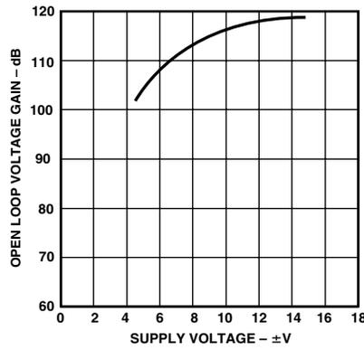
TPC 11. Open-Loop Voltage Gain vs. Supply Voltage
