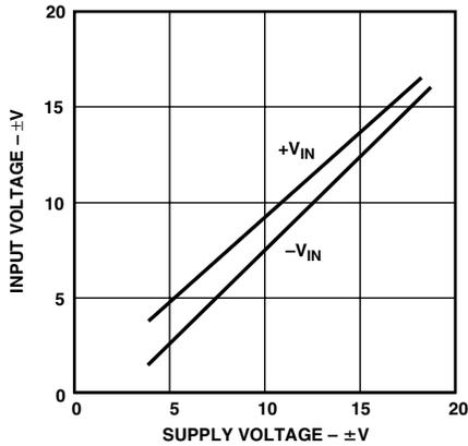
TPC 1. Input Voltage Range vs. Supply Voltage
