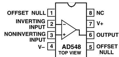
NOTE: PIN 4 CONNECTED TO CASE
