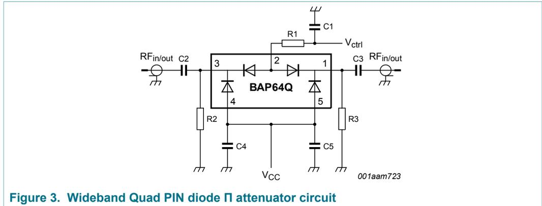
Figure 3. Wideband Quad PIN diode  $\Pi$  attenuator circuit
