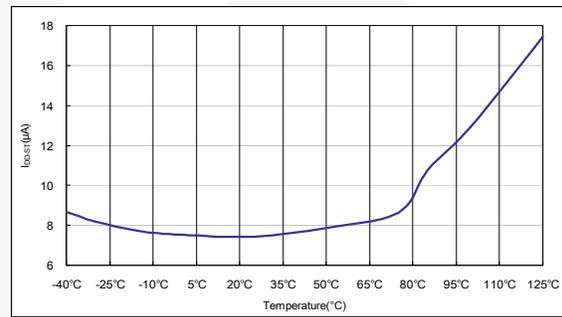
Figure 8. Startup Current
