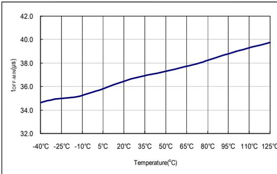
Figure 15. Minimum Off Time ( $V_{FB} = V_G$ )
