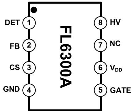
Figure 4. Pin Assignments
