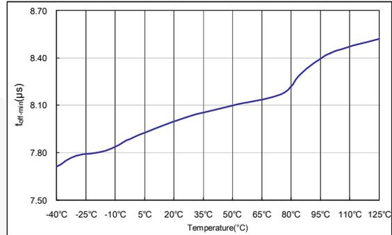
Figure 14. Minimum Off Time ( $V_{FB} > V_N$ )
