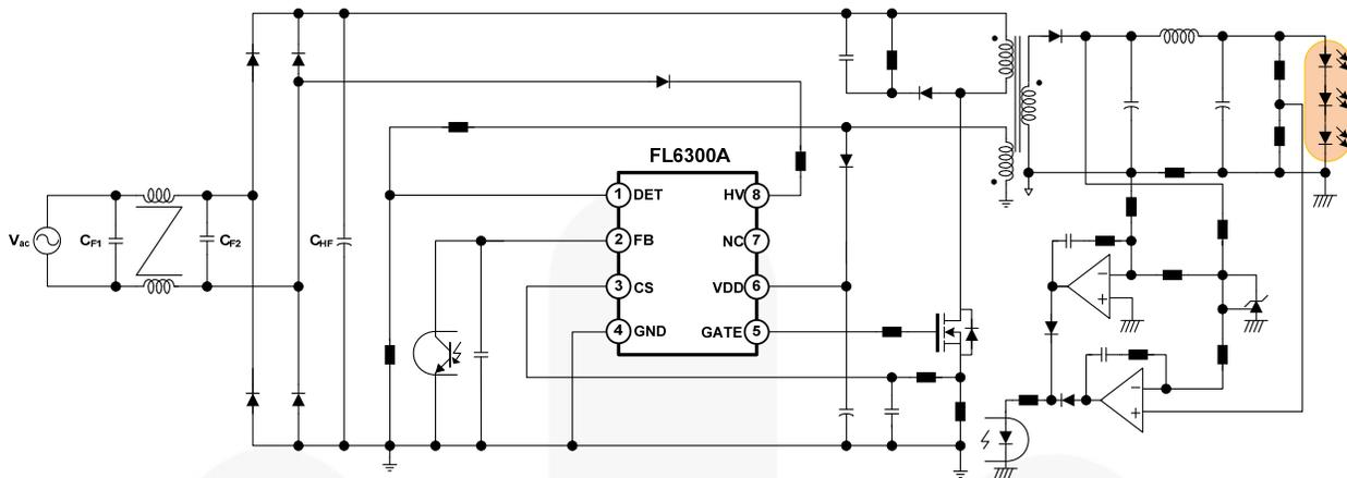
Figure 1. Typical Application Circuit for Flyback Converter
