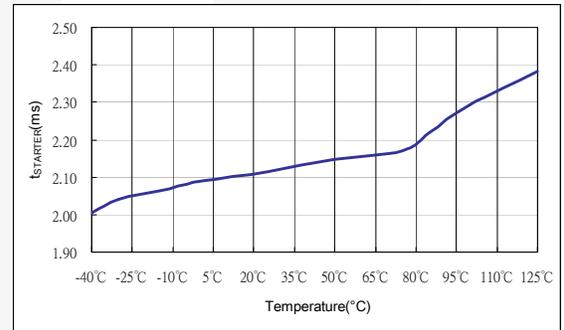
Figure 16. Start Timer ( $V_{FB} < V_G$ )
