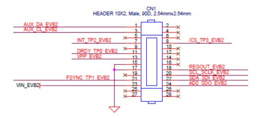
To connect to the Discovery Board you will need to connect these 5 pins on the Invensense EVB. Most Invensense EVBs do not populate the pins 1-4 and 25-28.
