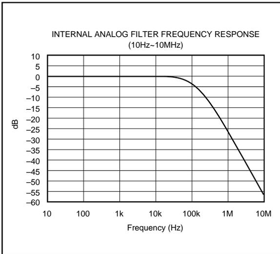
FIGURE 8. Low Pass Filter Wideband Frequency Response.
