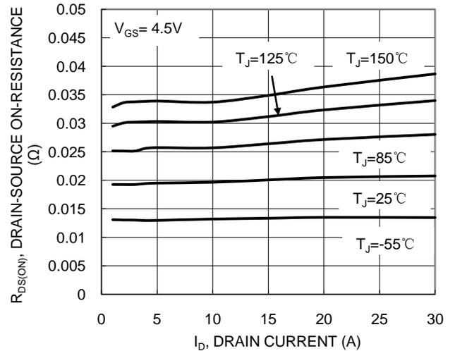
Figure 4. Typical On-Resistance vs. Drain Current and Temperature
