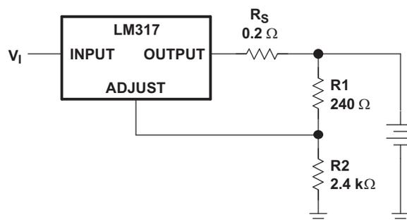
Figure 17. Battery-Charger Circuit
