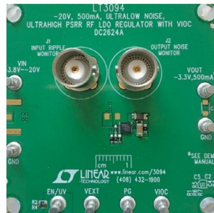
Figure 2. Demo circuit shows a tiny  $-3.3\ \text{V}$  solution.
