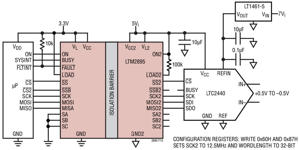
**Figure 13. Isolated System Measurement with 24-Bit SDM ADC**
