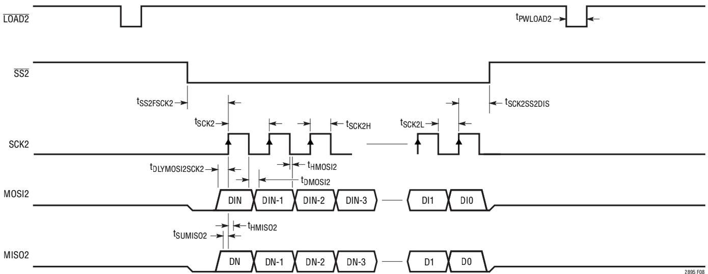
Figure 8. Logic Isolated Side Interface
