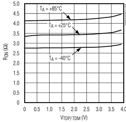
**DP/DM SHORT ON-RESISTANCE vs. SIGNAL VOLTAGE**
