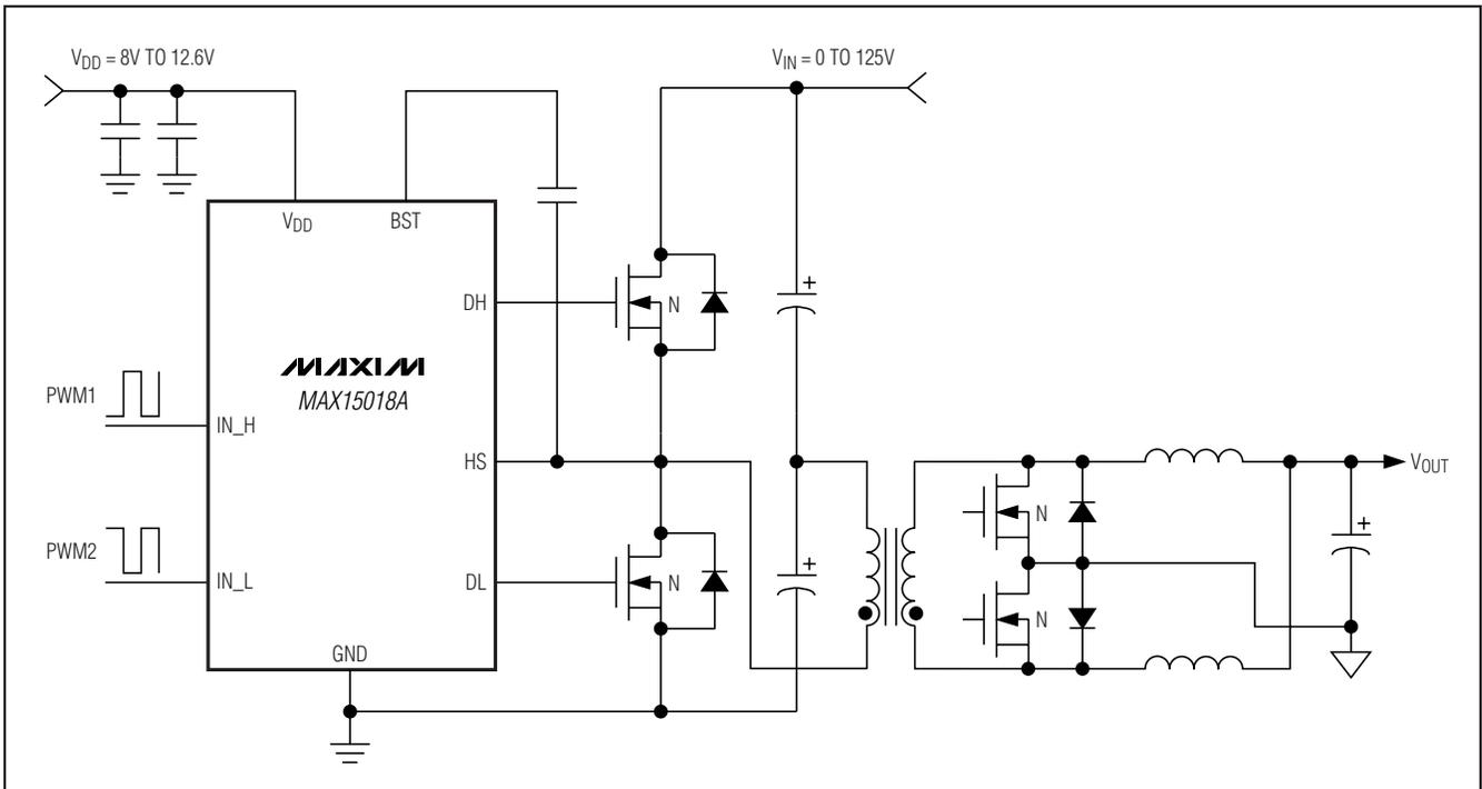
Figure 2. Half-Bridge Converter Application with Secondary-Side Synchronous Rectification
