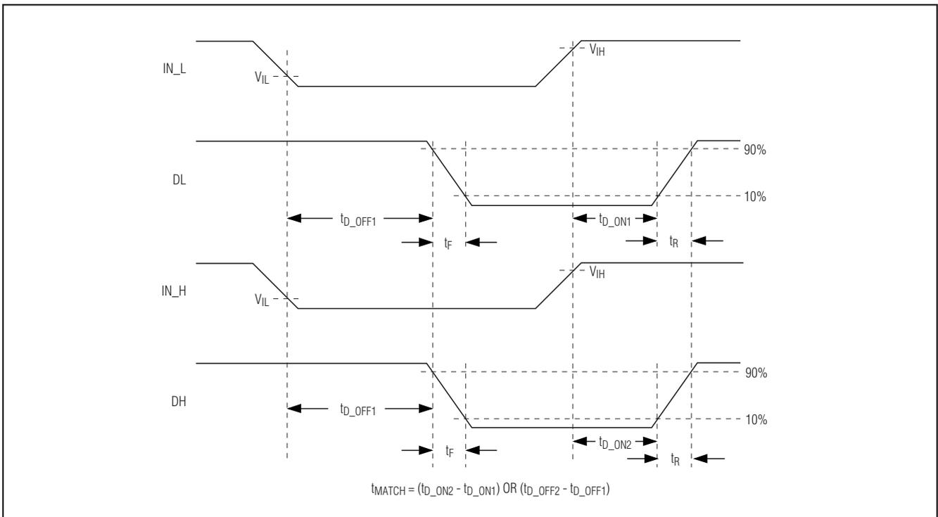
Figure 1. Timing Characteristics of Logic Inputs (MAX15018A/MAX15019A)
