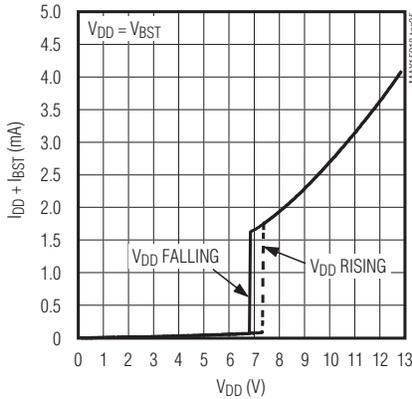
**INTERNAL BOOTSTRAP DIODE I-V CHARACTERISTICS**
