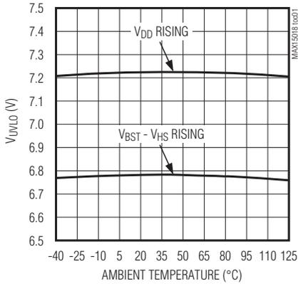
**V<sub>DD</sub> AND BST UNDERVOLTAGE LOCKOUT HYSTERESIS vs. TEMPERATURE**
