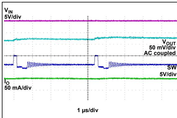
**FIGURE 2-26:** Switching Waveforms –  $I_{OUT} = 50 \text{ mA}$ , HLL.
