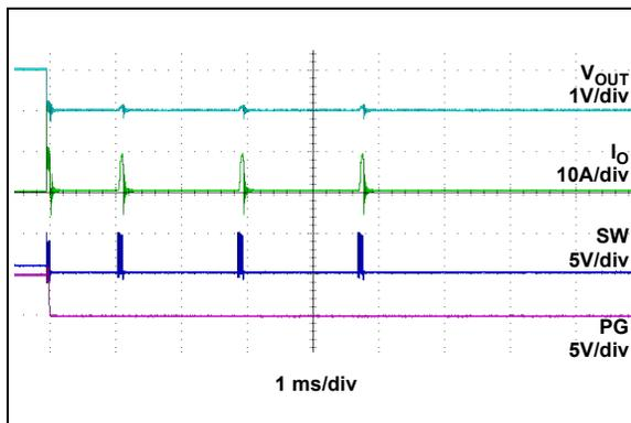
**FIGURE 2-25:** Hiccup Mode Short-Circuit Current Limit Response.
