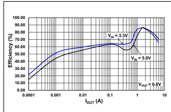
**FIGURE 2-6:** Efficiency vs. Load Current ( $V_{OUT} = 0.6V$ ).
