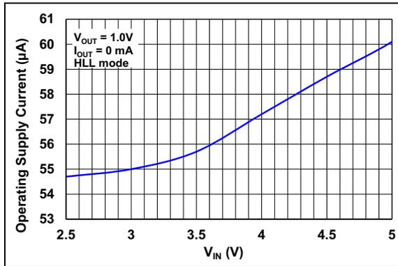
**FIGURE 2-1:** Operating Supply Current vs. Input Voltage, Switching.
