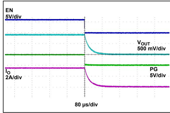
**FIGURE 2-21:**  $EN$  Turn-Off,  $R_{LOAD} = 0.3\Omega$ .
