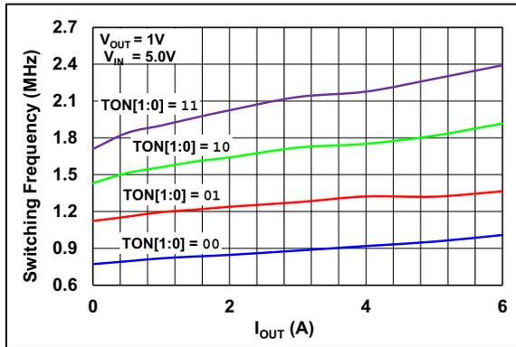
**FIGURE 2-13:** Switching Frequency vs.  $I_{OUT}$  ( $V_{OUT} = 1.0V$ ).
