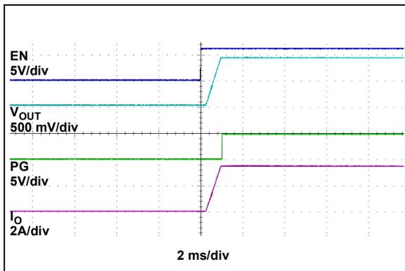
**FIGURE 2-20:**  $EN$  Turn-On,  $R_{LOAD} = 0.3\Omega$ .
