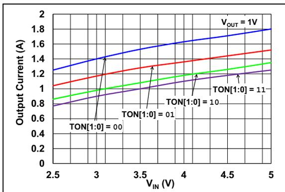
**FIGURE 2-9:** DCM/FPWM  $I_{OUT}$  Threshold vs.  $V_{IN}$ .
