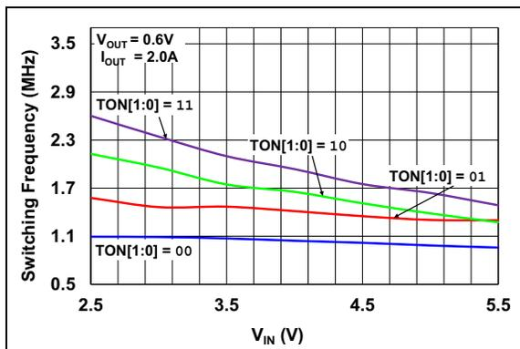
**FIGURE 2-15:** Switching Frequency vs.  $V_{IN}$  ( $V_{OUT} = 0.6V$ ).
