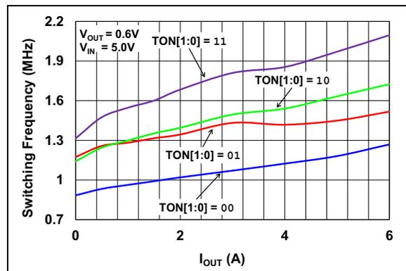
**FIGURE 2-12:** Switching Frequency vs.  $I_{OUT}$  ( $V_{OUT} = 0.6V$ ).
