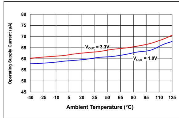
**FIGURE 2-4:** Operating Supply Current vs. Temperature, Switching.
