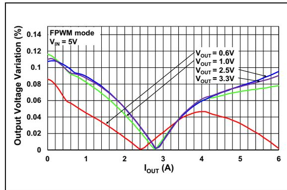
**FIGURE 2-11:** Load Regulation:  $V_{OUT}$  Voltage Variation vs.  $I_{OUT}$ .
