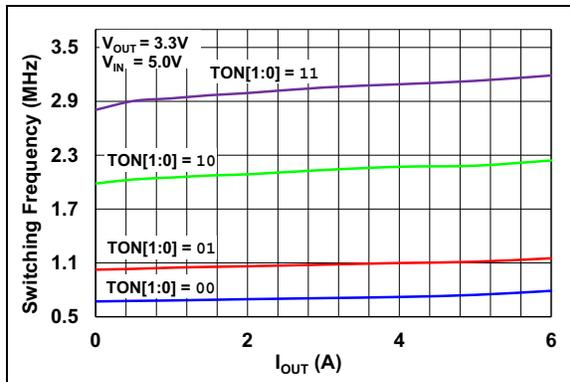
**FIGURE 2-14:** Switching Frequency vs.  $I_{OUT}$  ( $V_{OUT} = 3.3V$ ).
