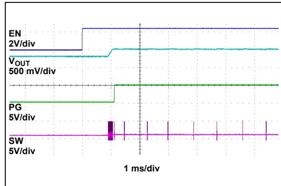
**FIGURE 2-22:**  $EN$  Turn-On into Pre-Biased Output ( $V_{pre-bias} = 0.8V$ ).
