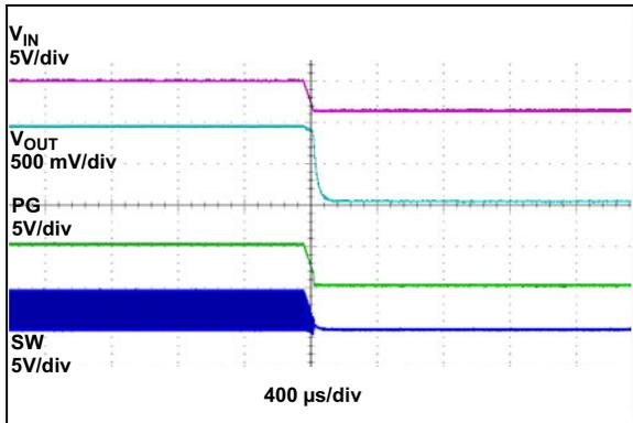
**FIGURE 2-19:**  $V_{IN}$  Turn-Off ( $EN = PV_{IN}$ ),  $R_{LOAD} = 0.3\Omega$ .
