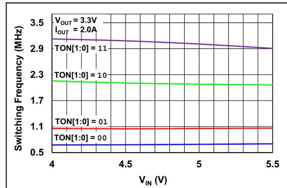
**FIGURE 2-17:** Switching Frequency vs.  $V_{IN}$  ( $V_{OUT} = 3.3V$ ).
