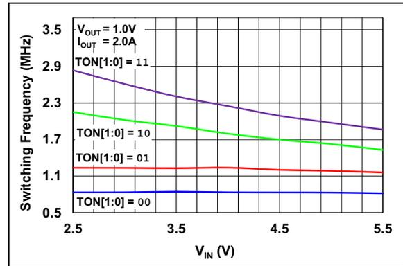
**FIGURE 2-16:** Switching Frequency vs.  $V_{IN}$  ( $V_{OUT} = 1.0V$ ).
