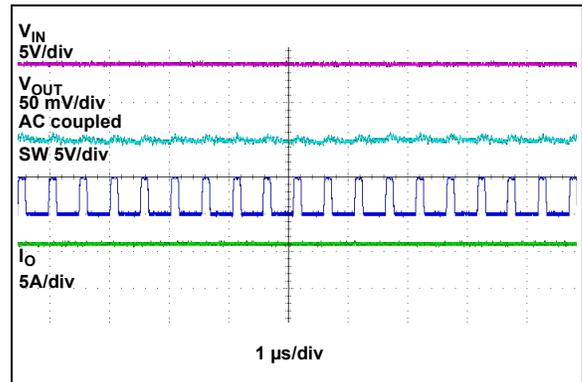
**FIGURE 2-27:** Switching Waveforms –  $I_{OUT} = 6A$ .
