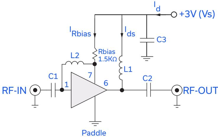
Fig 3. Recommended Application Circuit
