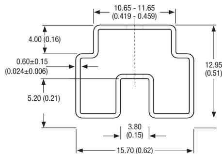
Tube material: Antistatic coated clear pvc
