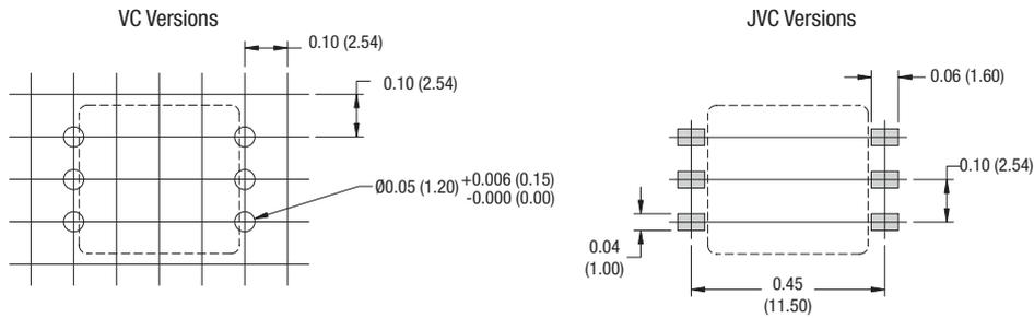
Unless otherwise stated all dimensions in mm (inches)  $\pm 0.25$  (0.01). All pins on a 2.54 (0.1) pitch and within  $\pm 0.25$  (0.01) of true position.
