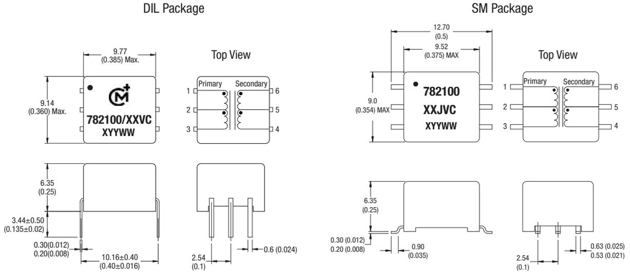
Unless otherwise stated all dimensions in mm (inches)  $\pm 0.25$  (0.01). All pins on a 2.54 (0.1) pitch and within  $\pm 0.25$  (0.01) of true position.
