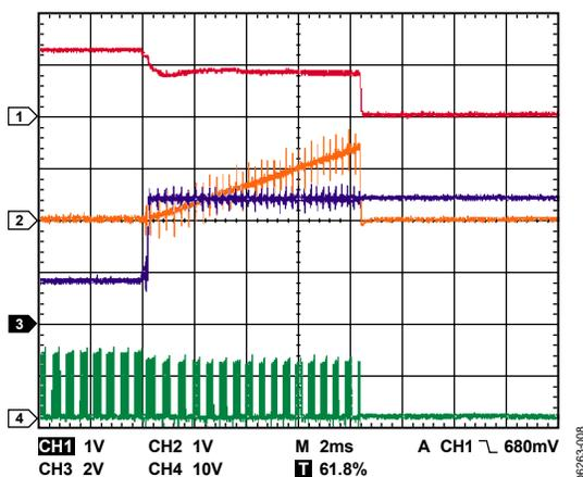
Figure 9. Overcurrent Latch-Off Waveforms
