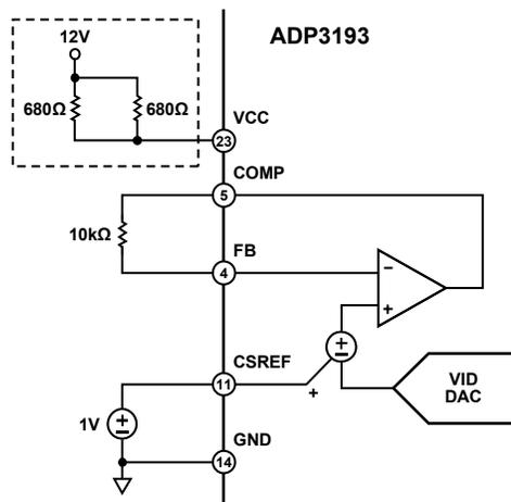
Figure 4. Positioning Voltage
