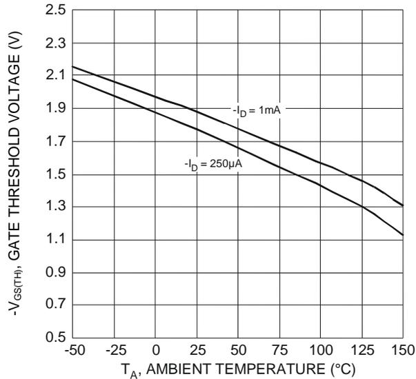
Figure 7 Gate Threshold Variation vs. Ambient Temperature
