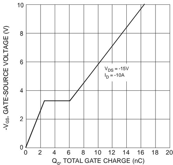
Figure 11 Gate-Charge Characteristics
