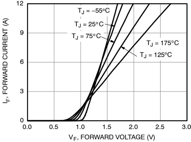
Figure 1. Forward Characteristics
