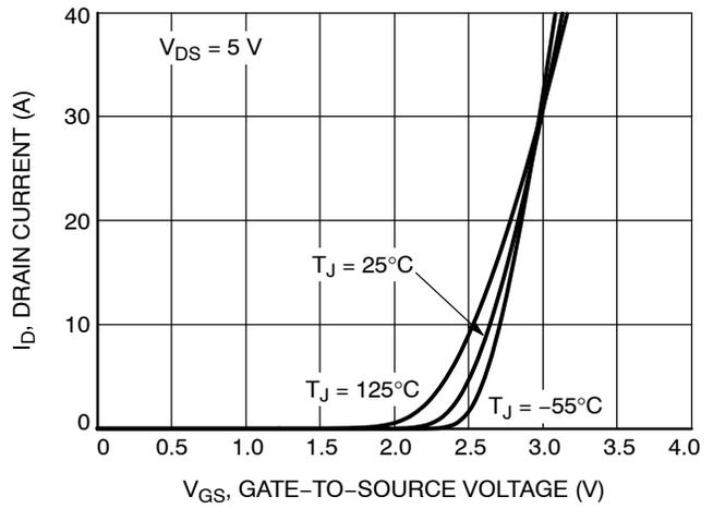
Figure 2. Transfer Characteristics
