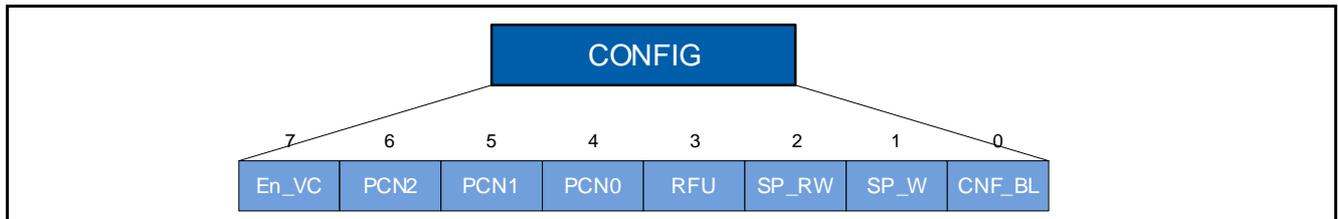
Figure 8 Configuration Byte
