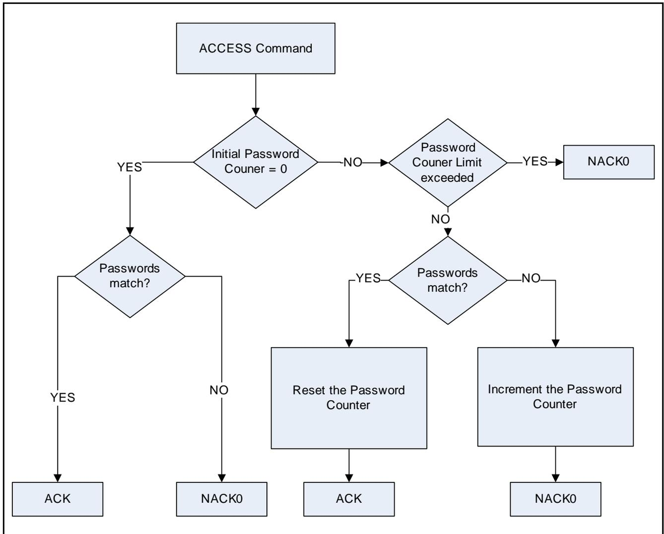
Figure 26 Flow Diagram of the ACS Command
