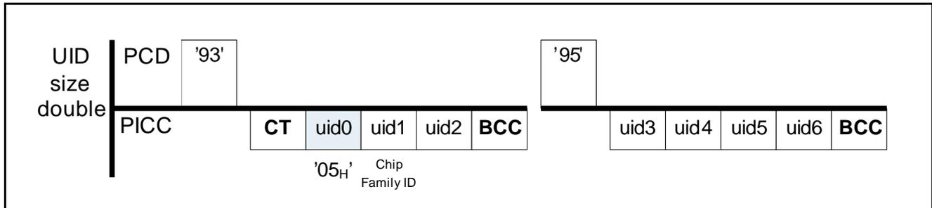
Figure 6 SLE 66R01P and SLE 66R01PN double-size UID
