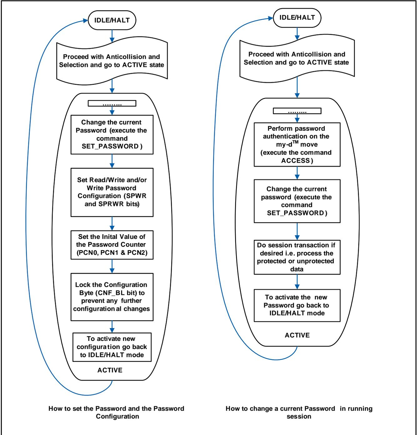
Figure 15 Password and Password Retry Counter configuration
