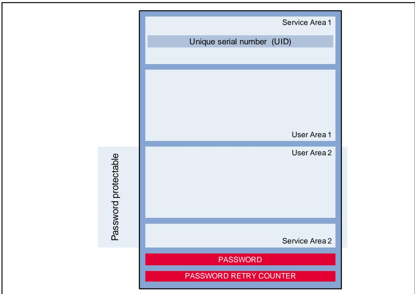
Figure 3 SLE 66R01P and SLE 66R01PN memory principle
