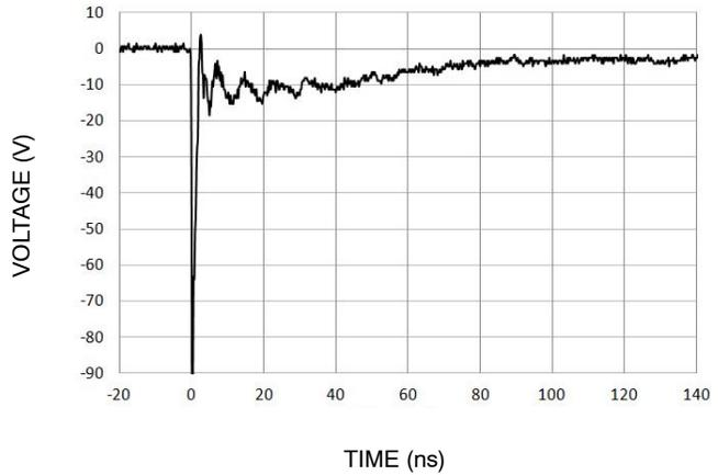
Figure 3. IEC61000-4-2 -8 kV Contact Clamping Voltage
