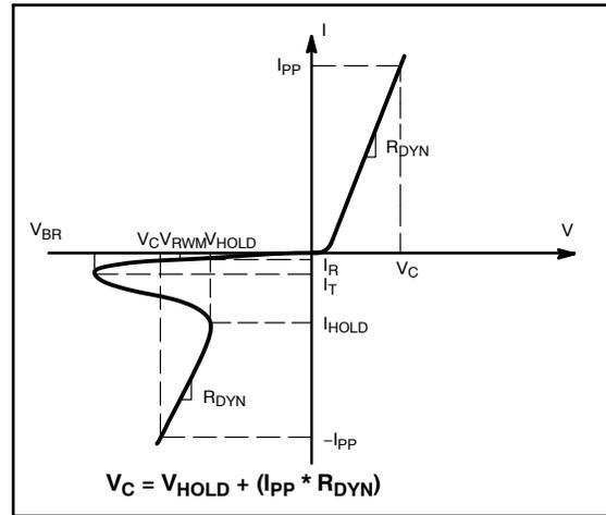
**ELECTRICAL CHARACTERISTICS** (T<sub>A</sub> = 25°C unless otherwise specified)
