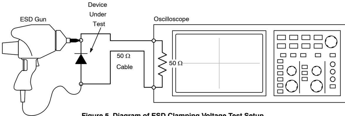
Figure 5. Diagram of ESD Clamping Voltage Test Setup
