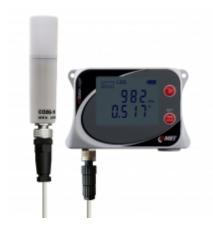
Battery powered datalogger with internal atmospheric pressure sensor and for external  $CO_2$  probe up to  $10\ 000ppm$ . In case of exceeded set limits alarms are indicated by LED, LCD and acoustically by built-in beeper.
