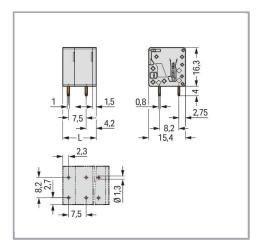
L = (pole no. - 1) x pin spacing + 6.5 mm
