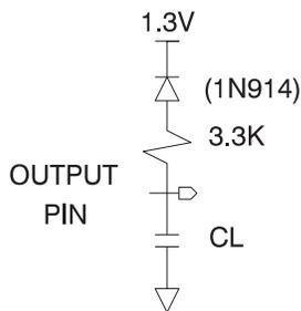
Note: 1.  $C_L = 100\text{pF}$  including jig capacitance, except for the -45 devices, where  $C_L = 30\text{pF}$ .
