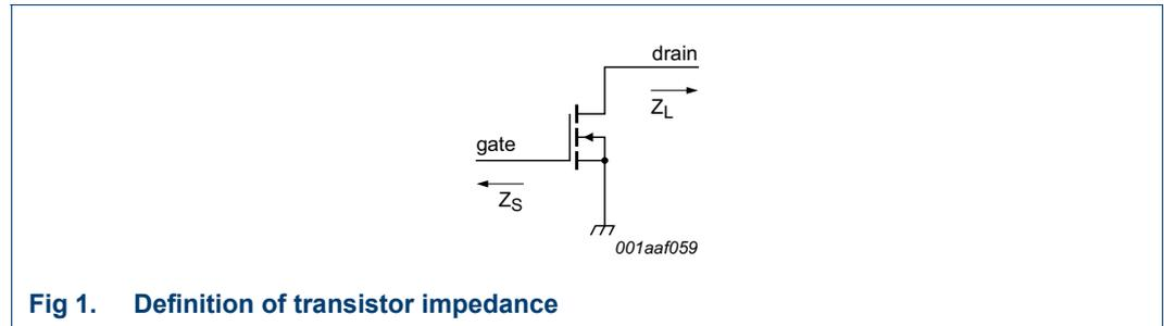
Fig 1. Definition of transistor impedance
