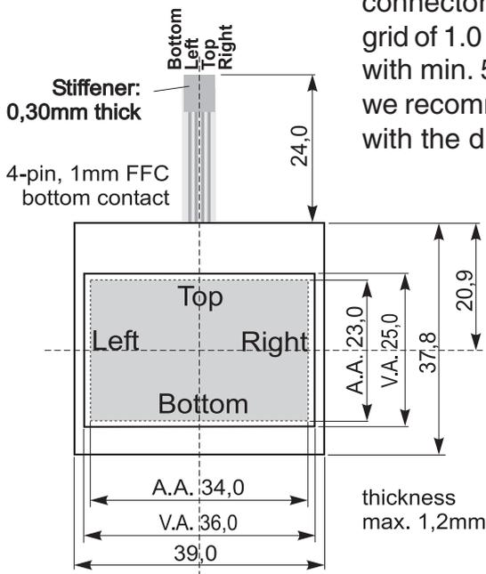
The pinout of the connecting cable is shown in the drawing. For connection there is a ZIF connector with pitch 1 mm, e.g. EA WF100-04S.
