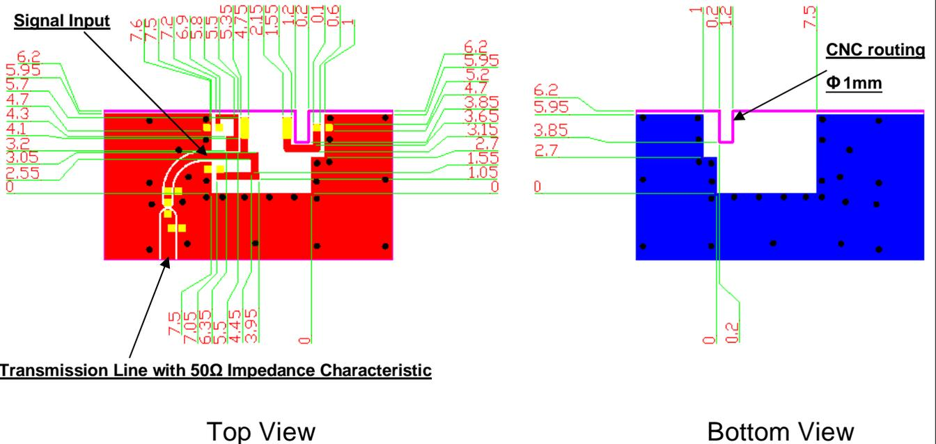
Transmission Line with 50Ω Impedance Characteristic
