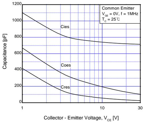
Fig 7. Capacitance Characteristics
