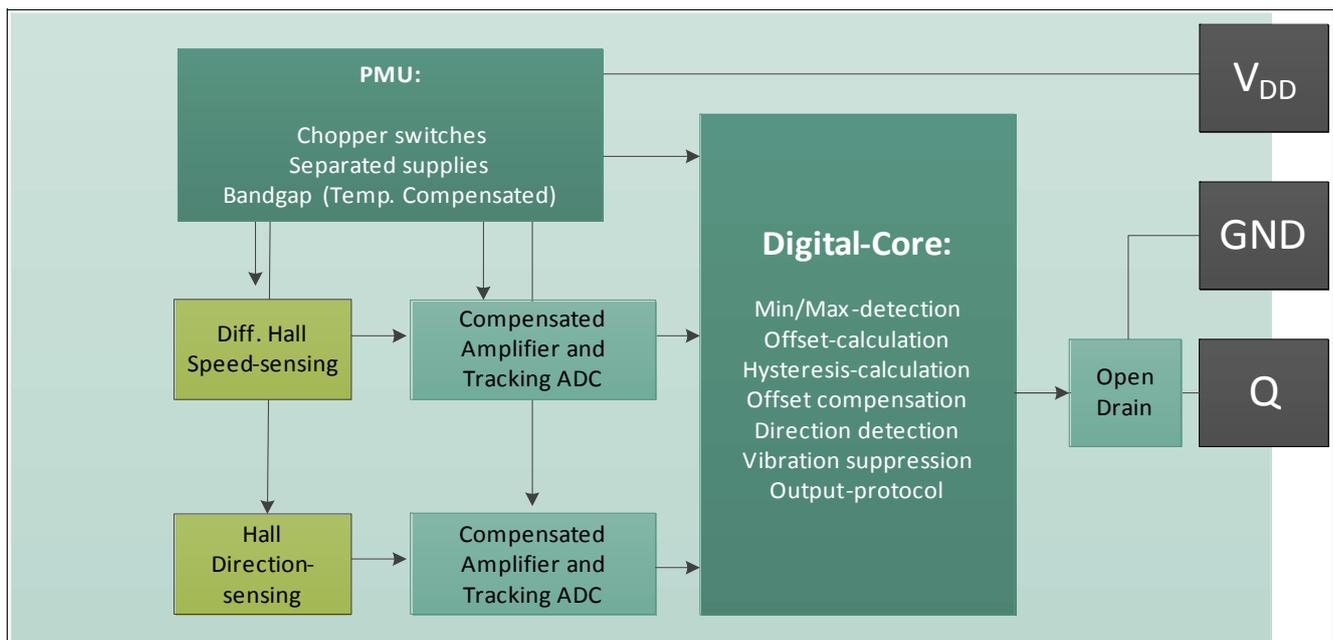
Figure 3 Block Diagram
