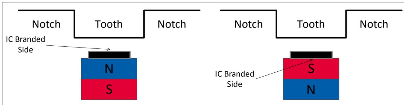
Figure 2 Definition of the Positive Magnetic Field Direction
