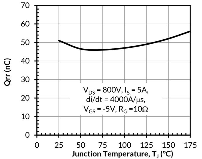
Figure 18. Reverse recovery charge  $Q_{rr}$  vs. junction temperature
