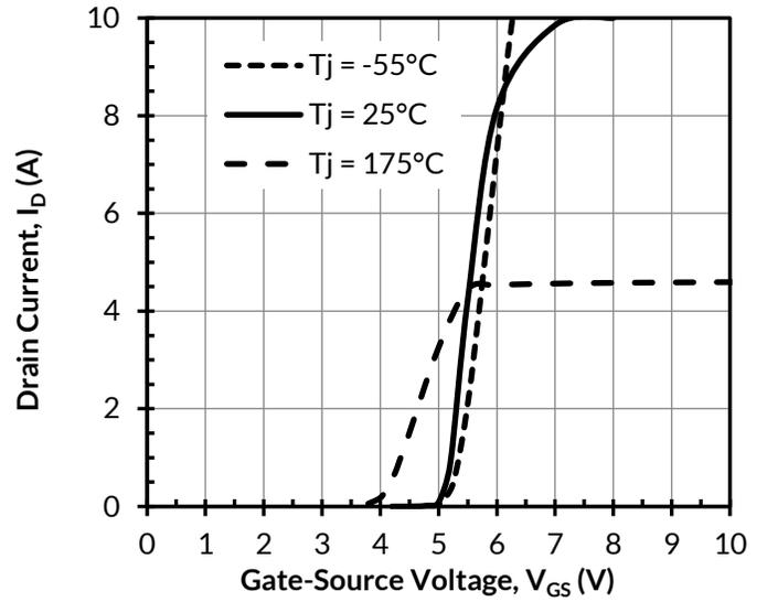
Figure 6. Typical transfer characteristics at  $V_{DS} = 5\text{V}$
