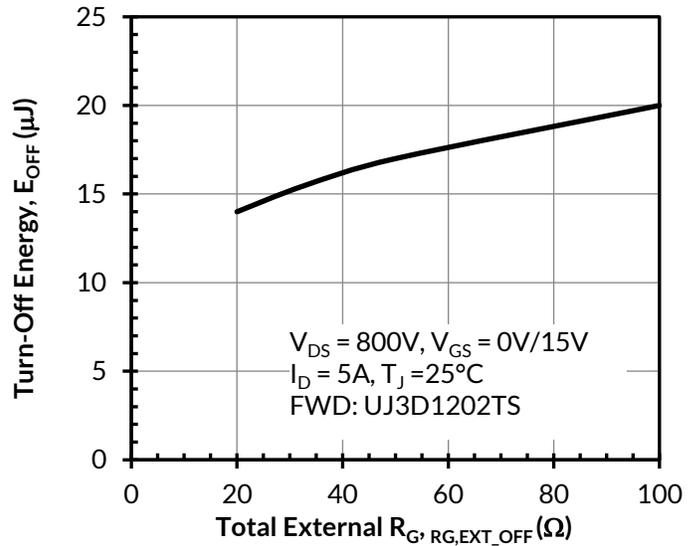
Figure 21. Clamped inductive switching turn-off energy vs.  $R_{G,EXT\_OFF}$
