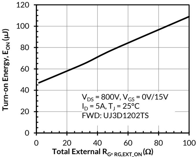
Figure 20. Clamped inductive switching turn-on energy vs.  $R_{G,EXT\_ON}$
