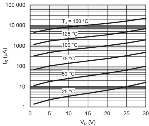
Fig. 2 - Typical Reverse Leakage Current vs. Reverse Voltage
