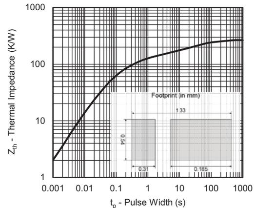
Fig. 4 - Typical Thermal Impedance vs. Time
