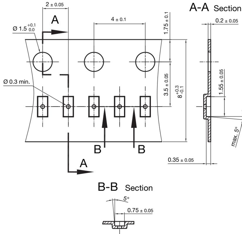
Cummulative tolerances of 10 sprocket holes is +/-0.2mm
