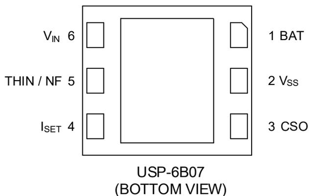
\*The dissipation pad for the USP-6B07 package should be solder-plated in recommended mount pattern and metal masking so as to enhance mounting strength and heat release.
