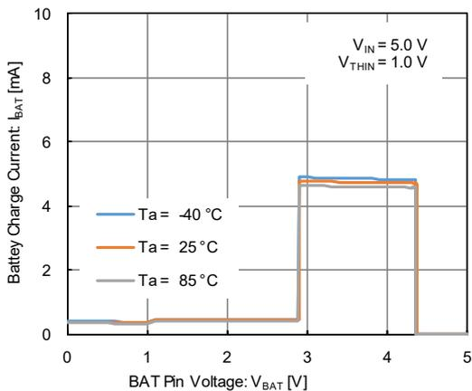
(4) Battery Charge Current vs. BAT Pin Voltage
