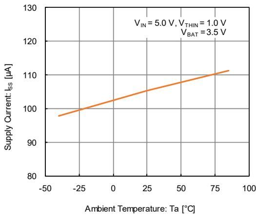
(8) Standby Current vs. Ambient Temperature
