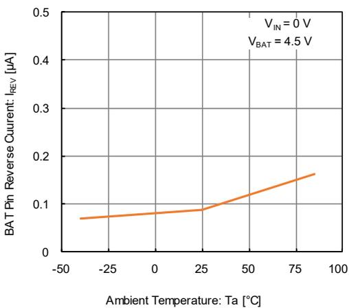
(12) BAT Pin Pull-down Current vs. Ambient Temperature
