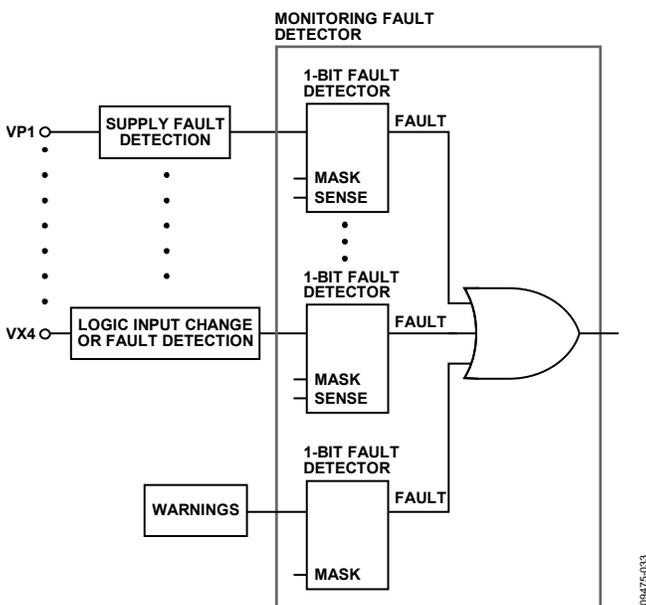
Figure 29. Monitoring Fault Detect or Block Diagram
