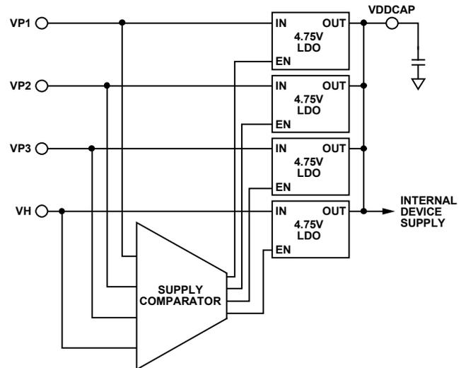
Figure 21. V<sub>DD</sub> Arbitrator Operation
