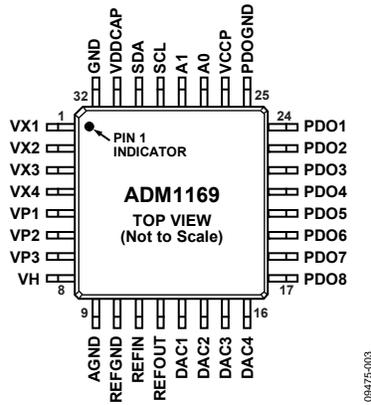
Figure 3. 32-Lead LQFP Pin Configuration
