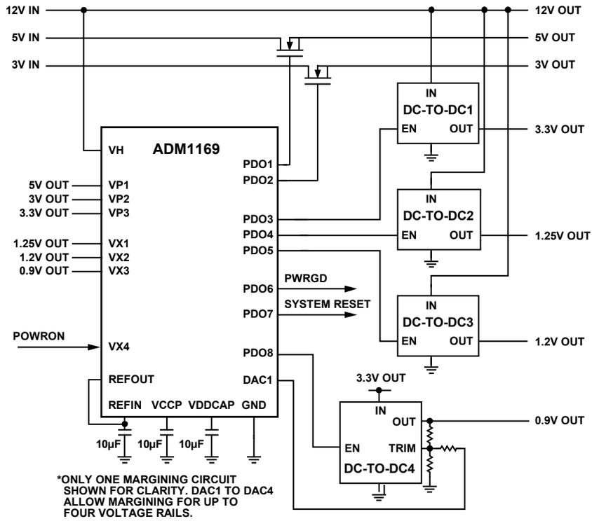
Figure 34. Applications Diagram
