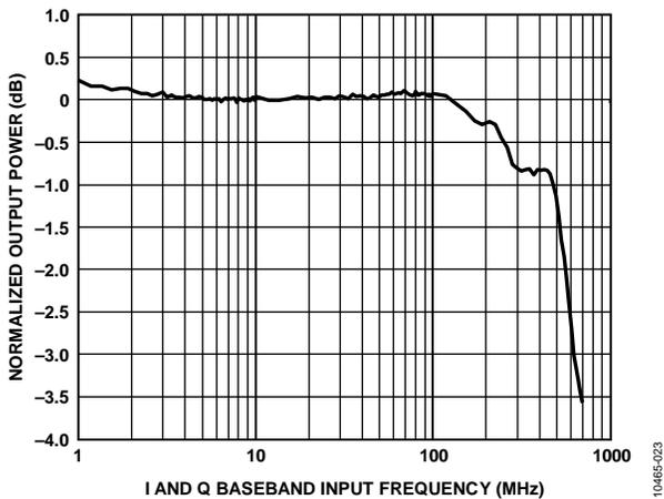
Figure 22. Normalized I and Q Input Bandwidth
