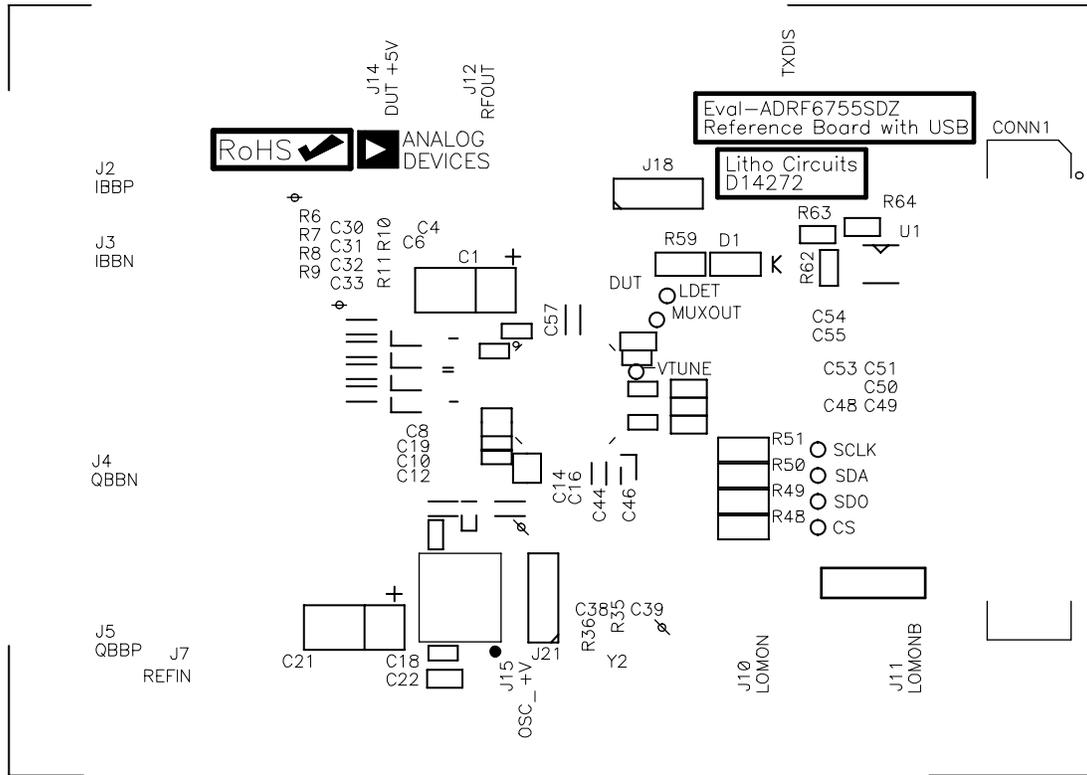
Figure 72. Evaluation Board, Top Side Component Placement
