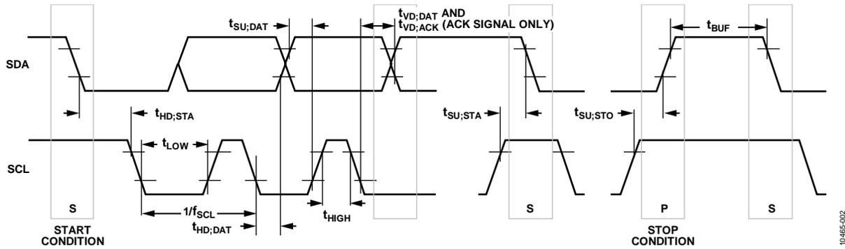
Figure 2. I<sup>2</sup>C Port Timing Diagram
