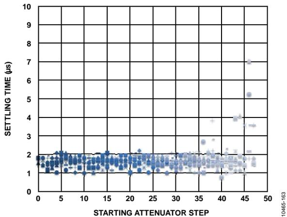
Figure 43. Attenuator Setting Time to 0.2 dB for Small Steps (1 dB to 6 dB) at Nominal Conditions
