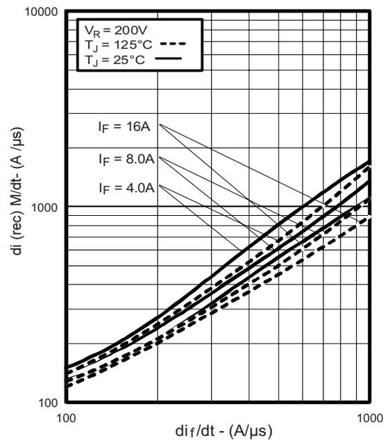
Fig. 8 - Typical  $di_{(rec)M}/dt$  vs.  $di_F/dt$  (Per Leg)
