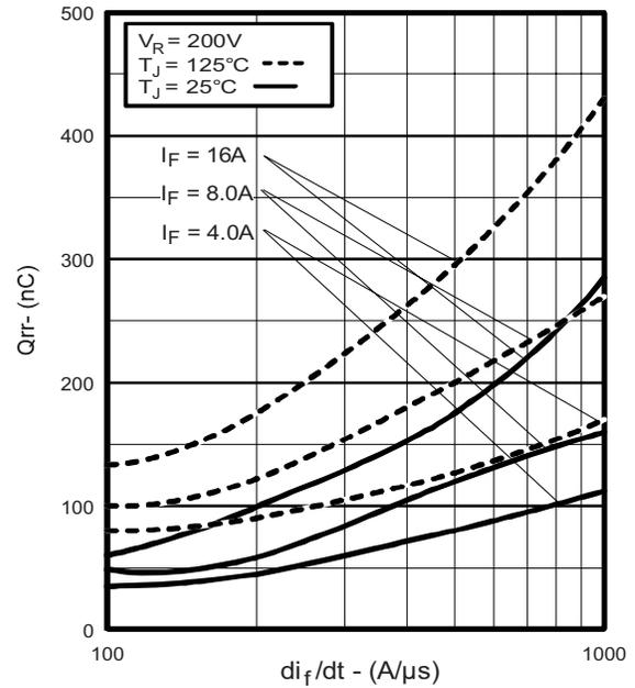
Fig. 7 - Typical Stored Charge vs.  $di_F/dt$  (Per Leg)
