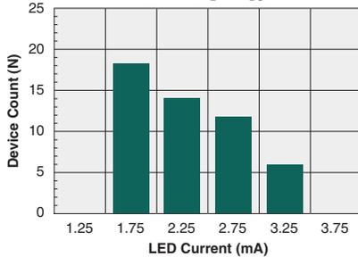
**Typical  $I_F$  for Switch Dropout**
