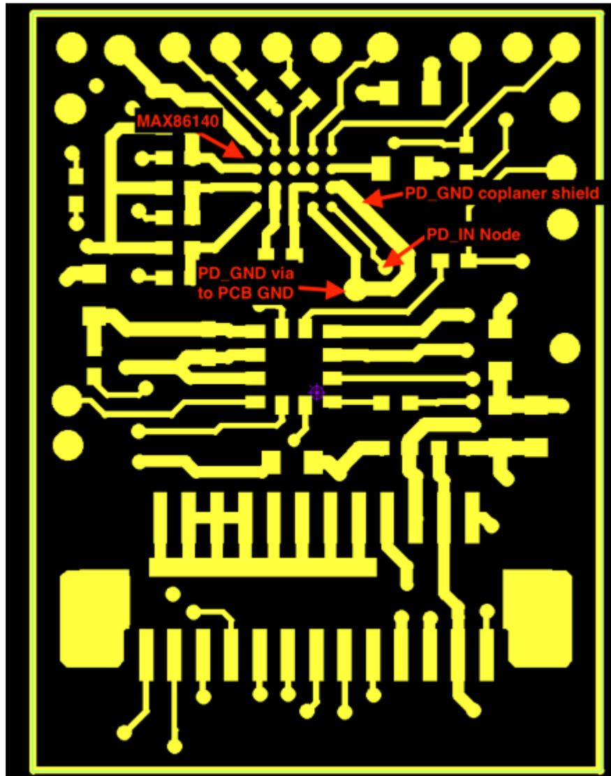
Figure 31. Example PCB Layout, Layer 1 (Top, MAX86140)
