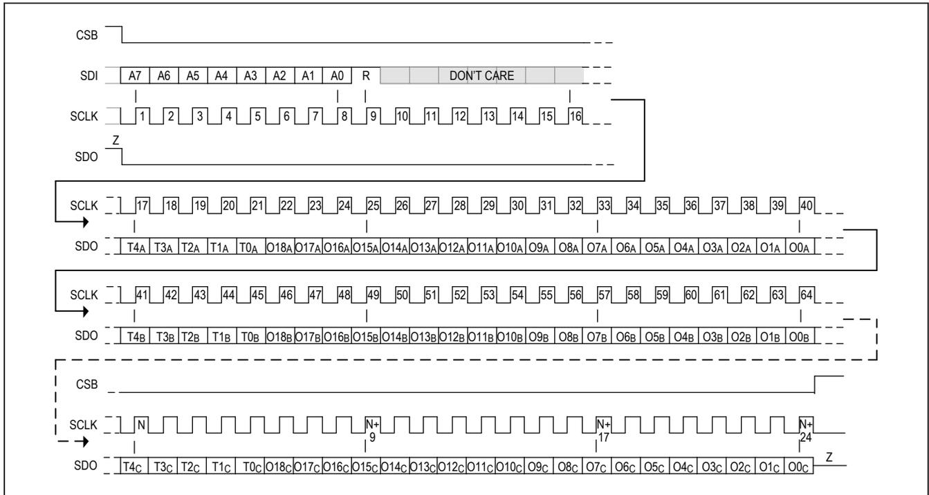
Figure 37. SPI FIFO Burst Mode Read Transaction
