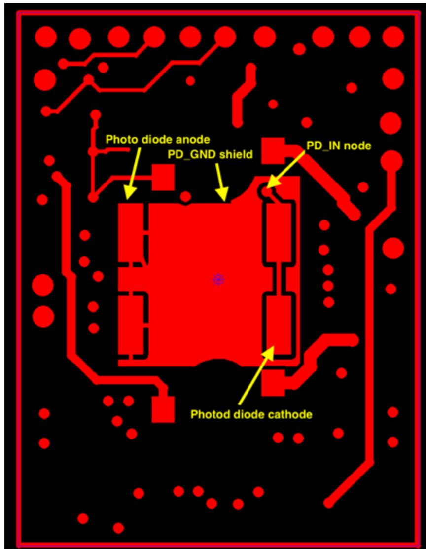
Figure 32. Example PCB Layout, Layer 6 (Bottom, Optical Layer)
