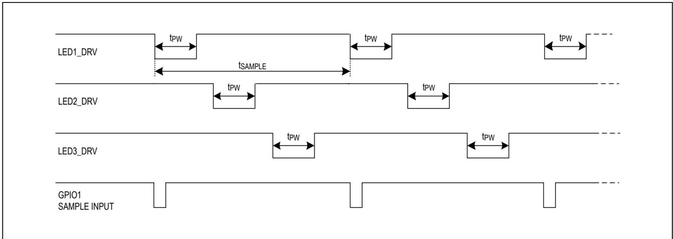
Figure 14. Timing Diagram for GPIO CTRL[3:0] 0011
