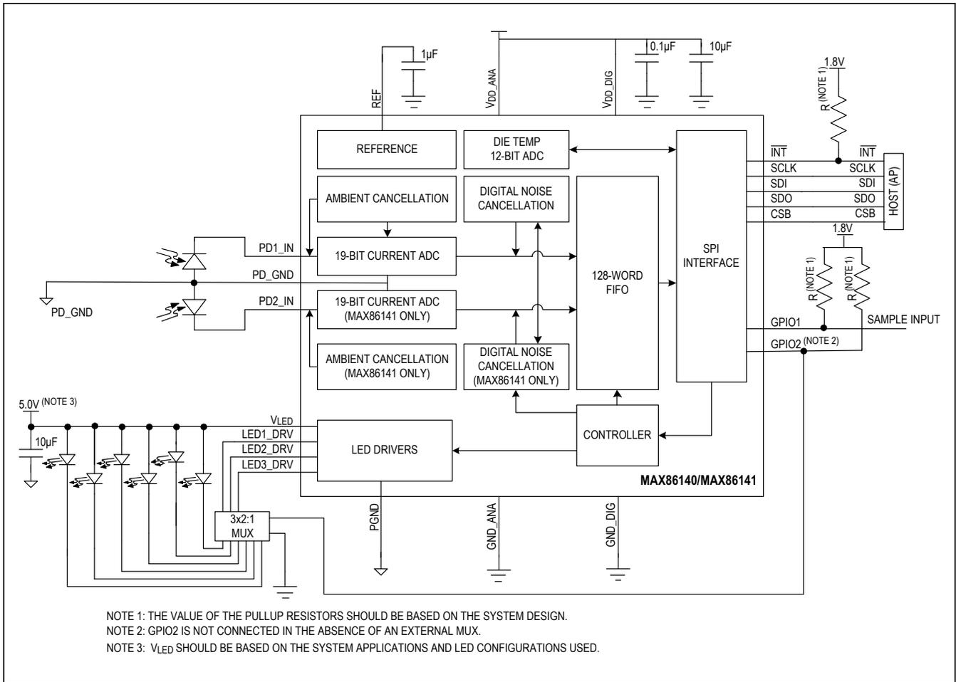
Figure 25. Block Diagram for GPIO CTRL[3:0] 1010
