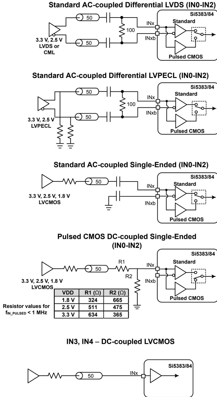
Figure 3.8. Termination of Differential and LVCMOS Input Signals
