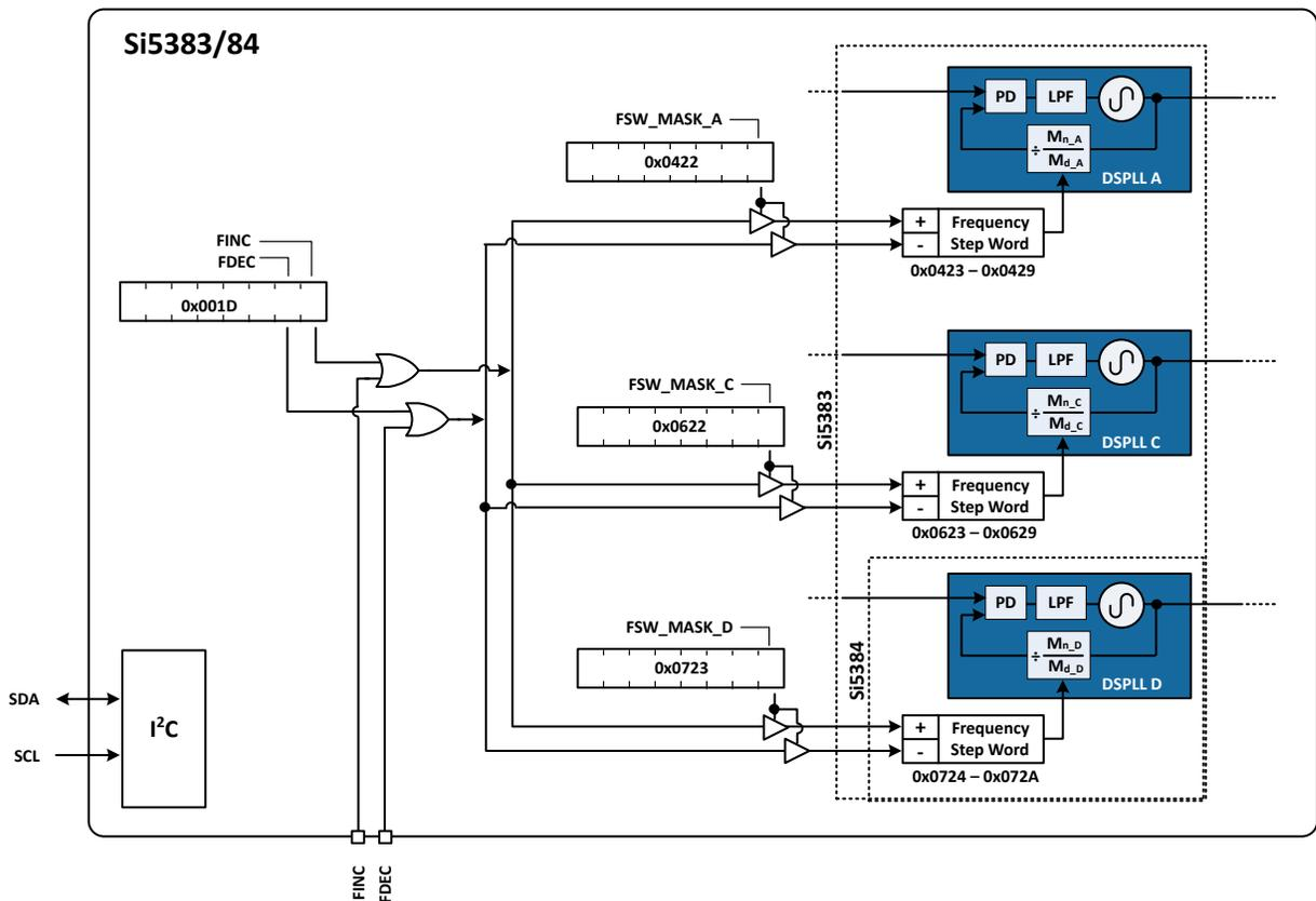
Figure 3.3. Controlling the DCO Mode By Pin Control
