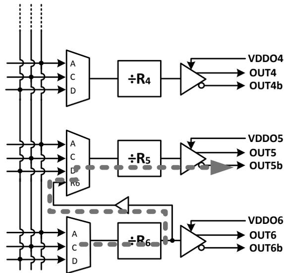
Figure 3.18. Generating a 1 Hz Output using the Si5383/84
