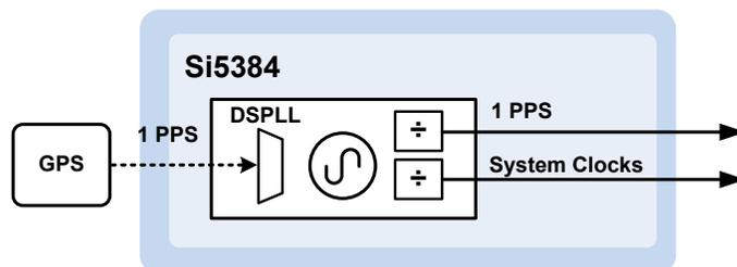
Figure 6.4. Si5384 as a 1 Hz/1 PPS Clock Multiplier
