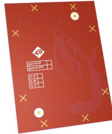
Where the Application PCB is shown to sit in Section 5.5, can house a small metal shield of the same size. This shield is used instead of, or underneath an Application PCB, to aid the on-board electronics in the prevention from potential RF or EMI signals.
