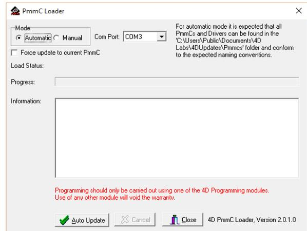
**Program Loader** is a GUI interface designed to download Applications to either Flash or RAM, useful for testing or production loading, without the need for Workshop4 itself.
