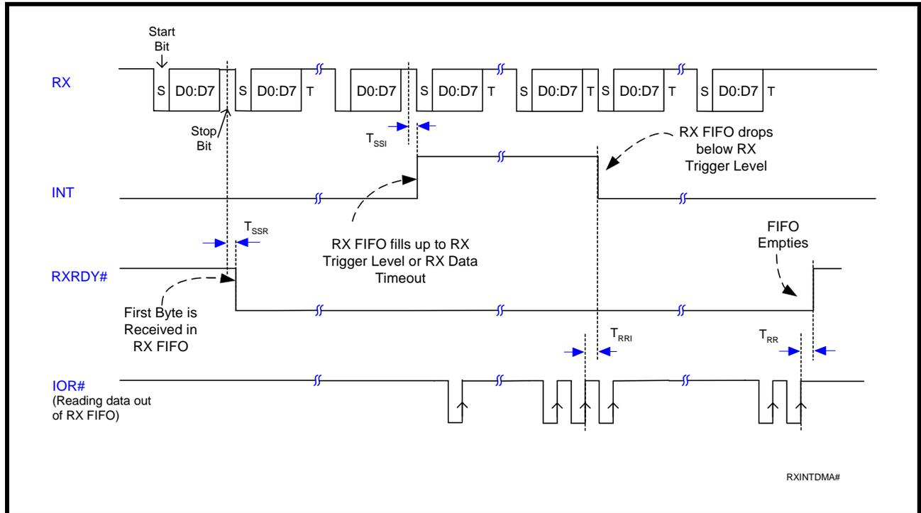
FIGURE 22. RECEIVE READY & INTERRUPT TIMING [FIFO MODE, DMA ENABLED] FOR CHANNELS A & B
