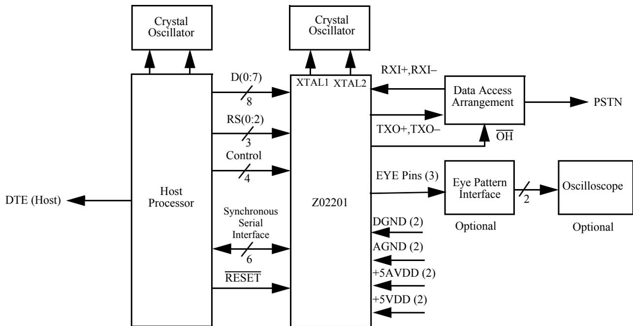
Figure 8. Modem Functional Interconnect Diagram
