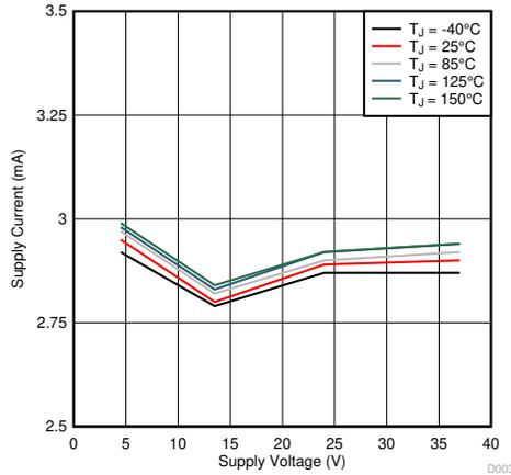
**Figure 6-4. Active Current ( $I_{VM}$ ) vs. Supply Voltage ( $V_{VM}$ )**
