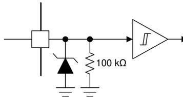
**Figure 7-2. Logic-Level Input**
