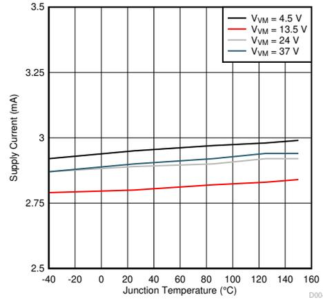
**Figure 6-5. Active Current ( $I_{VM}$ ) vs. Junction Temperature**
