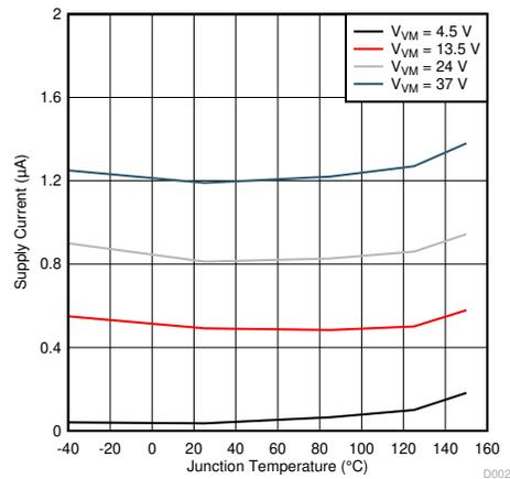
**Figure 6-3. Sleep Current ( $I_{VM0}$ ) vs. Junction Temperature**
