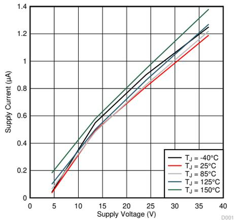
**Figure 6-2. Sleep Current ( $I_{VM0}$ ) vs. Supply Voltage ( $V_{VM}$ )**
