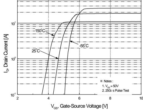
**Figure 2. Transfer Characteristics**
