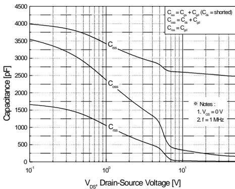
**Figure 5. Capacitance Characteristics**
