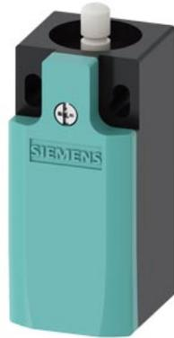
Position switch Plastic 31 mm according to EN 50047 Increased corrosion protection Device connection 1 x (M20 x 1.5) 1 NO/1 NC quick action contacts Rounded plunger functional at -40 °C Shock and vibration test according to EN 61373, Category 1B
