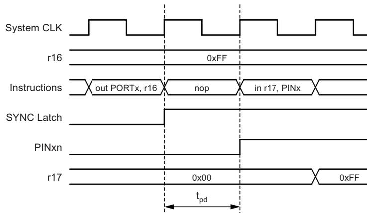
The following code example shows how to set port B pins 0 and 1 high, 2 and 3 low, and define the port pins from 4 to 5 as input with a pull-up assigned to port pin 4. The resulting pin values are read back again, but as previously discussed, a *nop* instruction is included to read back the value recently assigned to some of the pins.
