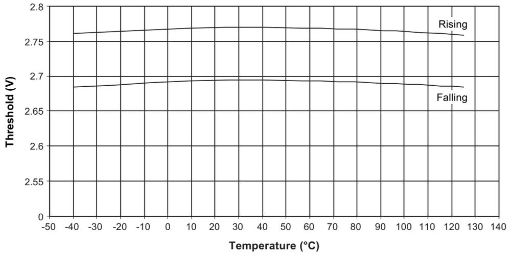
Figure 22-33. BOD Thresholds versus Temperature (BODLEVEL Is 1.8V)
