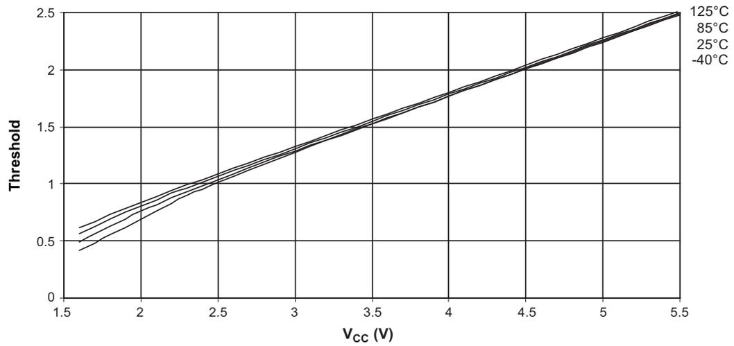
Figure 22-27. I/O Pin Input Hysteresis versus  $V_{CC}$
