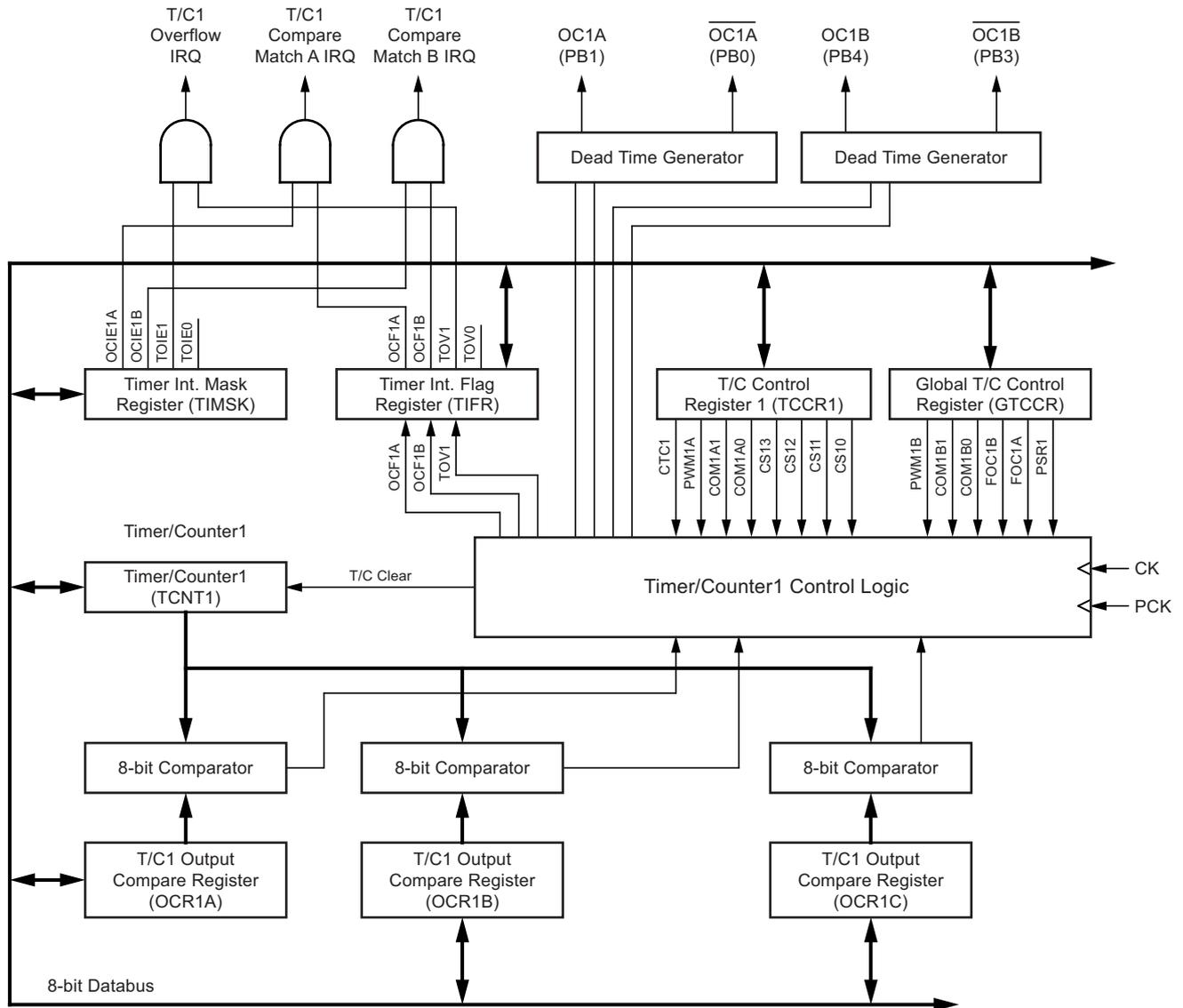
Three status flags (overflow and compare matches) are found in the Timer/Counter interrupt flag register - TIFR. control signals are found in the Timer/Counter control registers TCCR1 and GTCCR. The interrupt enable/disable settings are found in the Timer/Counter interrupt mask register - TIMSK.
