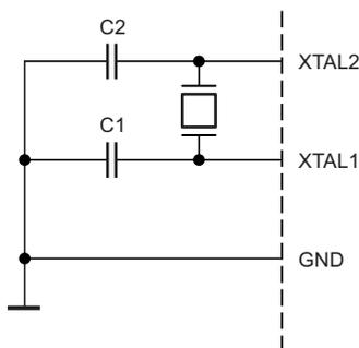
The oscillator can operate in three different modes, each optimized for a specific frequency range. The operating mode is selected by the fuses CKSEL3..1 as shown in [Table 5-3](#).
