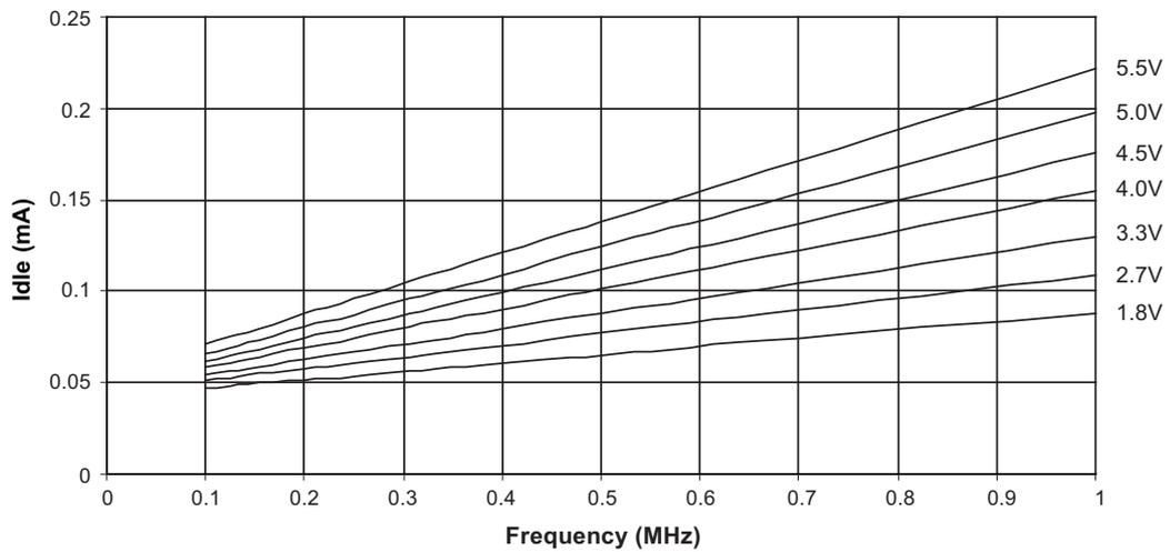
**Figure 22-7. Idle Supply Current versus Frequency (1 to 20MHz)**
