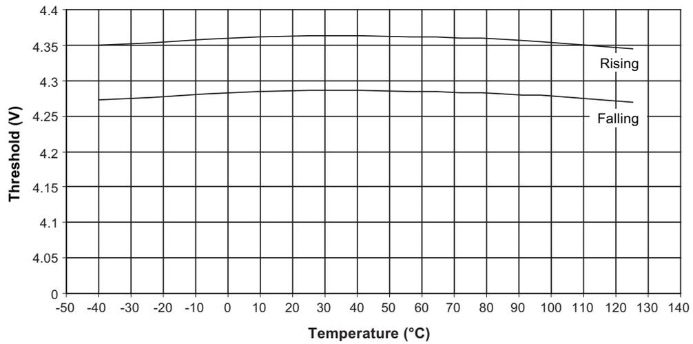
Figure 22-32. BOD Thresholds versus Temperature (BODLEVEL Is 2.7V)
