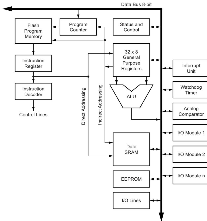
In order to maximize performance and parallelism, the AVR<sup>®</sup> uses a harvard architecture – with separate memories and buses for program and data. Instructions in the program memory are executed with a single level pipelining. While one instruction is being executed, the next instruction is pre-fetched from the program memory. This concept enables instructions to be executed in every clock cycle. The program memory is in-system reprogrammable flash memory.
