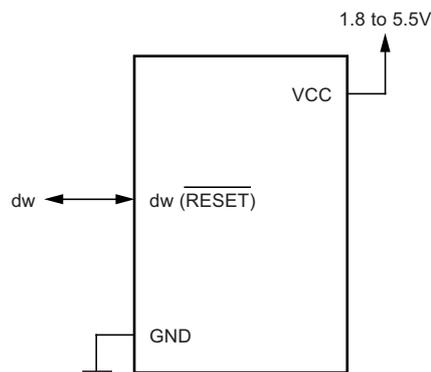
Figure 18-1 shows the schematic of a target MCU, with debugWIRE enabled, and the emulator connector. The system clock is not affected by debugWIRE and will always be the clock source selected by the CKSEL fuses.
