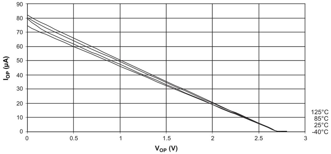
Figure 22-15. I/O Pin Pull-Up Resistor Current versus Input Voltage ( $V_{CC} = 5.0V$ )
