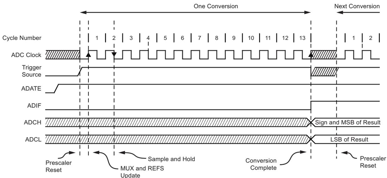
**Figure 17-7. ADC Timing Diagram, Free Running Conversion**
