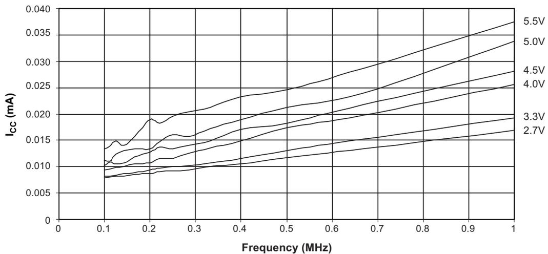
**Figure 22-2. Active Supply Current versus Frequency (1 to 20MHz)**
