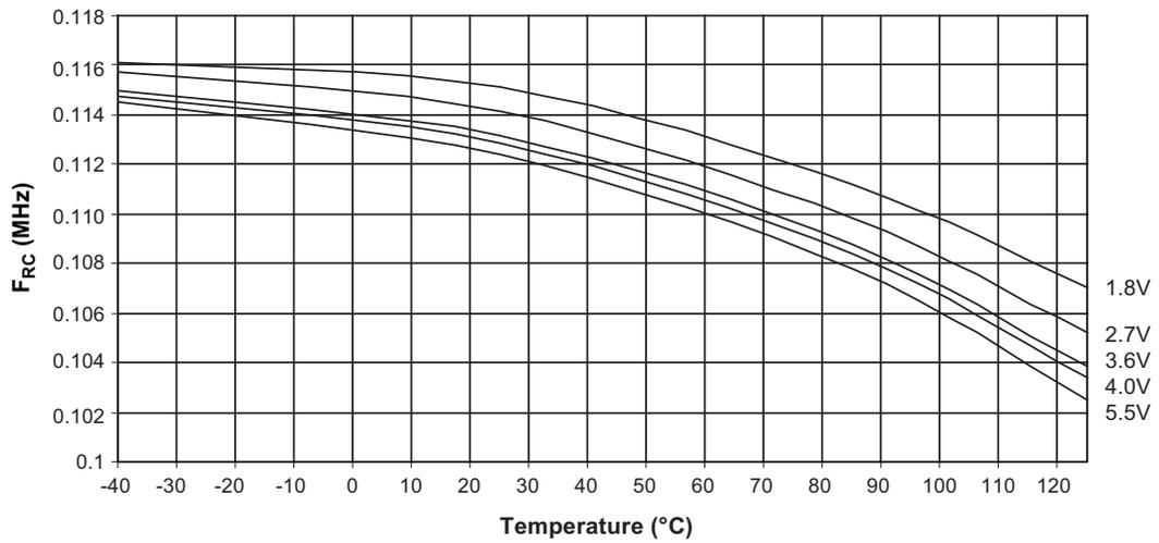
**Figure 22-36. Calibrated 8MHz RC Oscillator Frequency versus Temperature**
