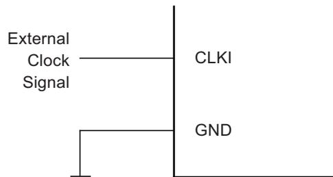
When this clock source is selected, start-up times are determined by the SUT fuses as shown in [Table 5-9](#).
