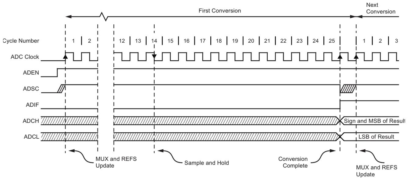
**Figure 17-5. ADC Timing Diagram, Single Conversion**
