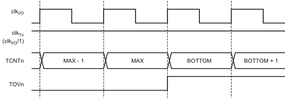
Figure 11-9 shows the same timing data, but with the prescaler enabled.
