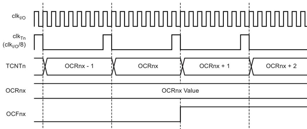
Figure 11-11 shows the setting of OCF0A and the clearing of TCNT0 in CTC mode and fast PWM mode where OCR0A is TOP.
