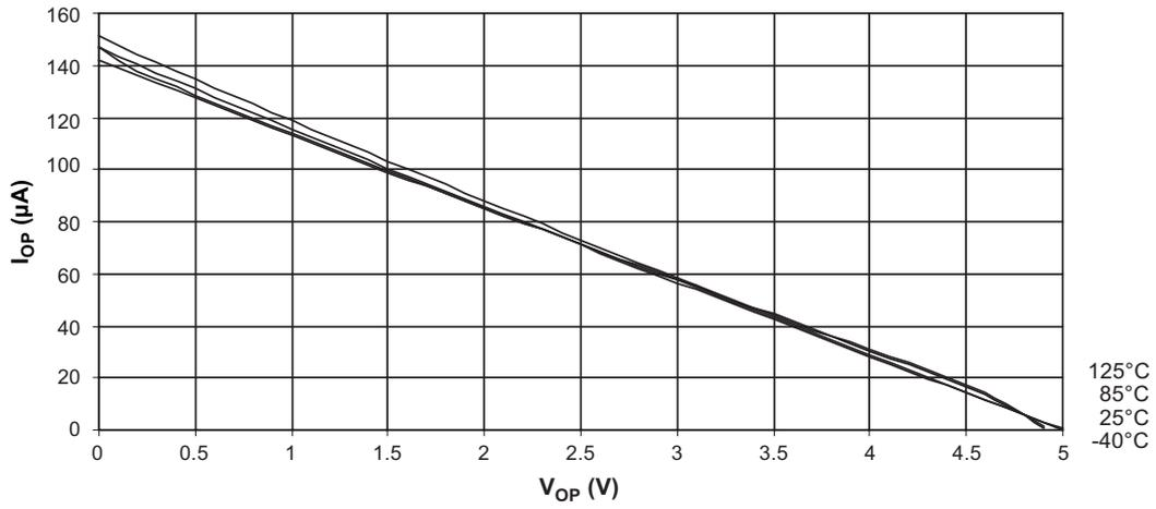
Figure 22-16. Reset Pull-Up Resistor Current versus Reset Pin Voltage ( $V_{CC} = 1.8V$ )
