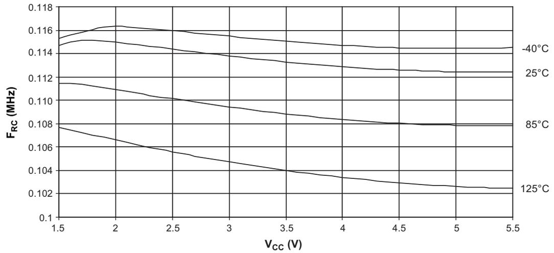
Figure 22-35. Watchdog Oscillator Frequency versus Temperature
