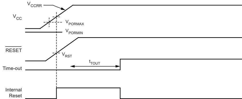
**Figure 7-3. MCU Start-up, RESET Extended Externally**
