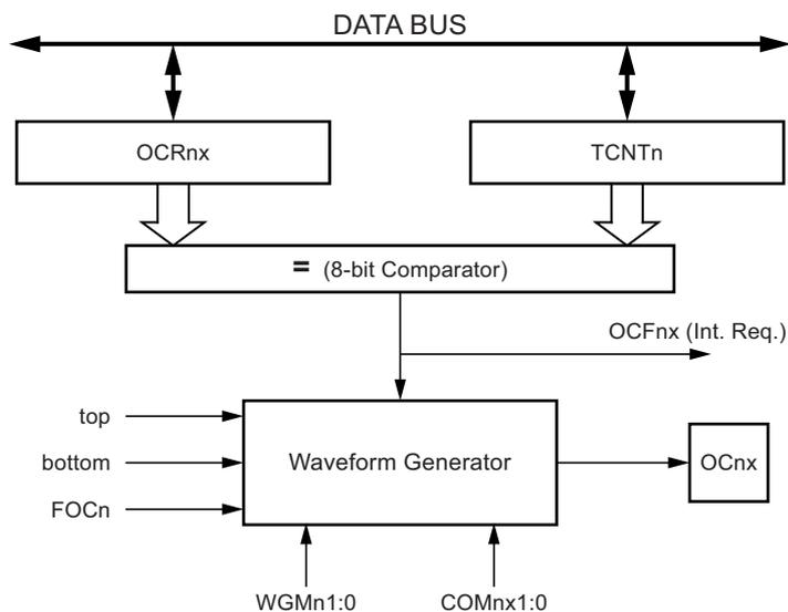
The OCR0x registers are double buffered when using any of the pulse width modulation (PWM) modes. For the normal and clear timer on compare (CTC) modes of operation, the double buffering is disabled. The double buffering synchronizes the update of the OCR0x compare registers to either top or bottom of the counting sequence. The synchronization prevents the occurrence of odd-length, non-symmetrical PWM pulses, thereby making the output glitch-free.
