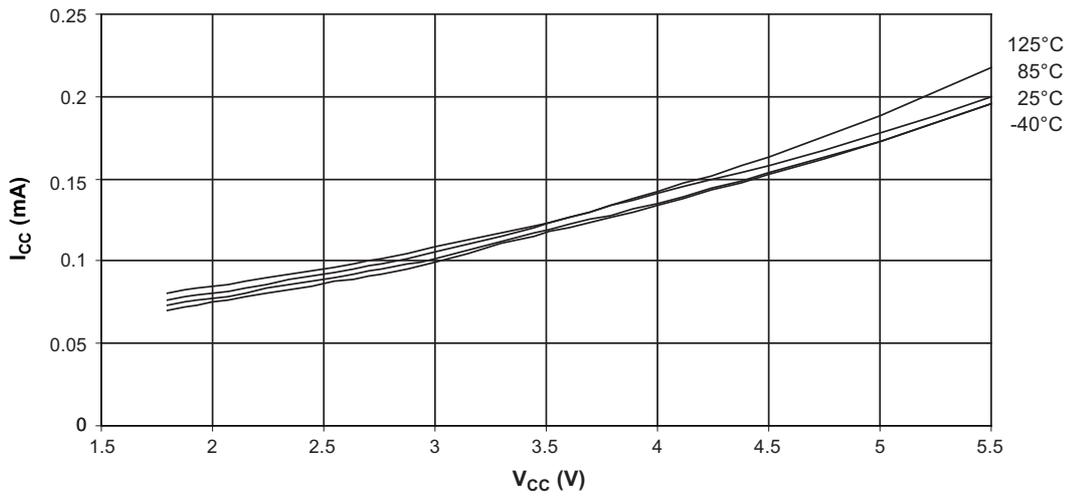
**Figure 22-9. Idle Supply Current versus V<sub>CC</sub> (Internal RC Oscillator, 1MHz)**
