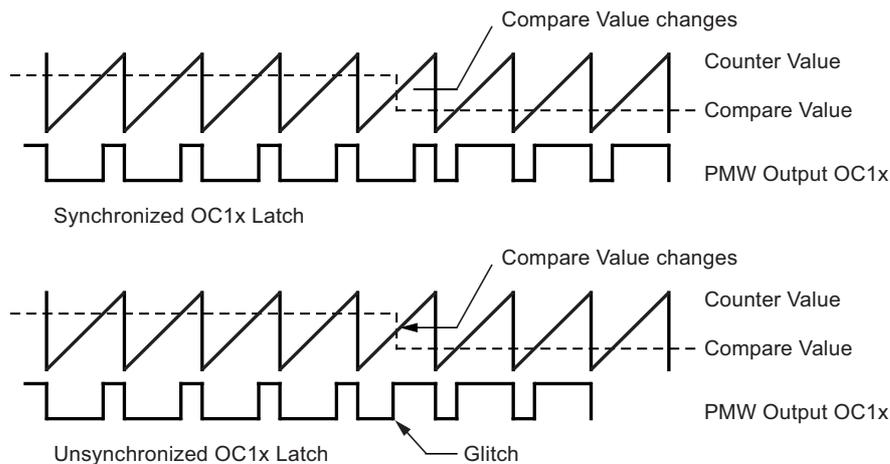
During the time between the write and the latch operation, a read from OCR1A or OCR1B will read the contents of the temporary location. This means that the most recently written value always will read out of OCR1A or OCR1B.
