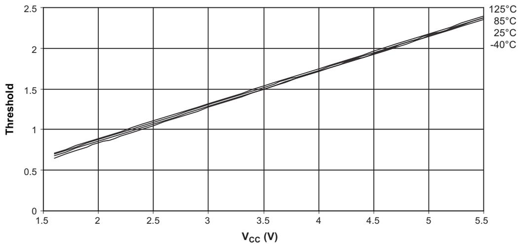
Figure 22-30. Reset Input Pin Hysteresis versus  $V_{CC}$
