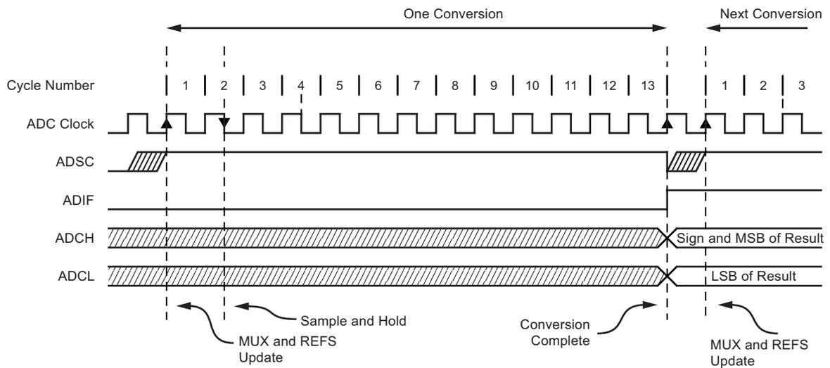
**Figure 17-6. ADC Timing Diagram, Auto Triggered Conversion**
