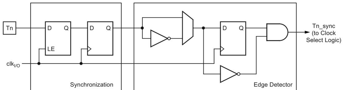
The synchronization and edge detector logic introduces a delay of 2.5 to 3.5 system clock cycles from an edge has been applied to the T0 pin to the counter is updated.
