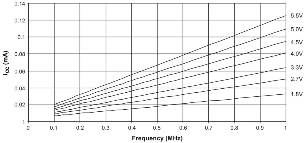
Figure 22-42. Reset Supply Current versus  $V_{CC}$  (1 to 24MHz, Excluding Current through the Reset Pull-up)
