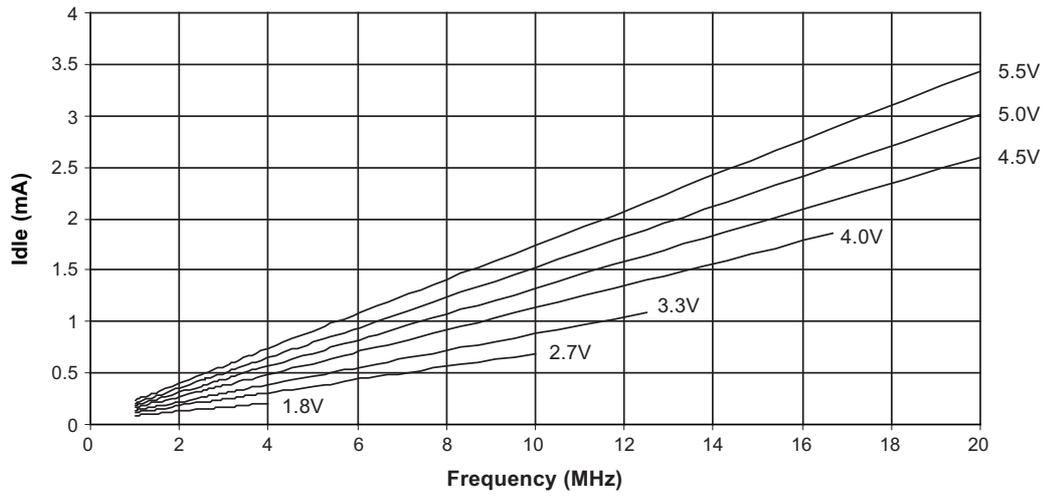
**Figure 22-8. Idle Supply Current versus V<sub>CC</sub> (Internal RC Oscillator, 128kHz)**
