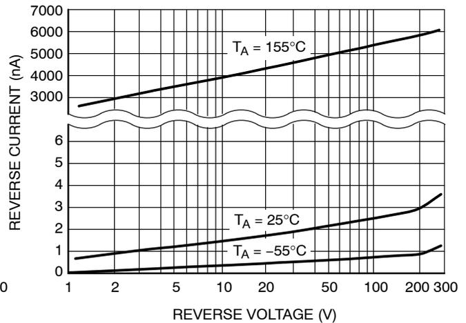
**Figure 3. Reverse Leakage**
